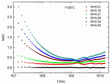
Figure 3. The spectra of the normalized attenuation coefficient (NAC) depending on the volumetric moisture content of the soil sample (W) at a temperature of  $T=25 \,^{\circ}$  C.
