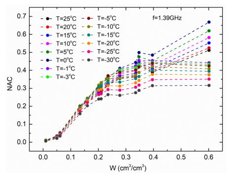
Figure 7. Normalized attenuation coefficient (NAC) as a function of soil sample moisture (W) for various temperatures at a 170 frequency of f=1.39 GHz.
