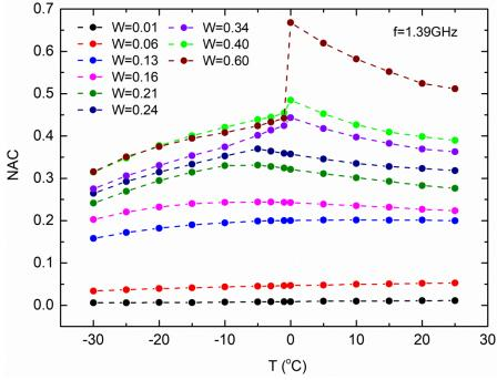
Figure 5. Normalized attenuation coefficient (NAC) depending on the temperature of the soil sample (T) for various moisture at a frequency of f=1.39 GHz.
