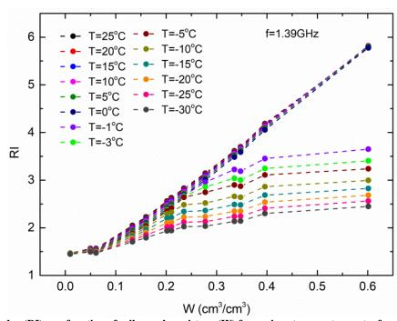
Figure 6. Refractive index (RI) as a function of soil sample moisture (W) for various temperatures at a frequency of f=1.39 GHz.
