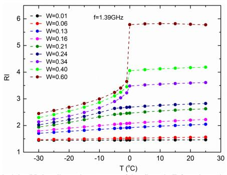
Figure 4. The refractive index (RI) depending on the temperature of the soil sample (T) for various moisture at a frequency of f=1.39 GHz.
