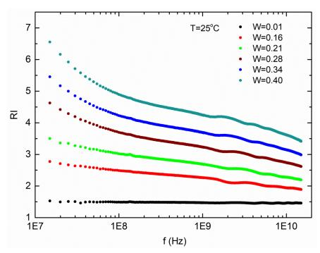
Figure 2. The spectra of the refractive index (RI) depending on the volumetric moisture content of the soil sample (W) at a temperature of T=25 ° C. Volumetric moisture has dimension W=[cm³cm⁻³] here and in other Figures.
