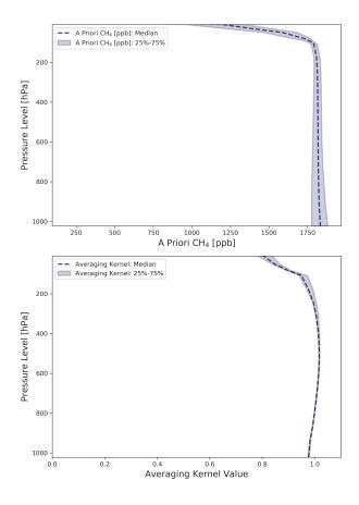
**Figure 1.** The average  $CH_4$  a priori profile used in the retrievals along with the 25-75% variation (top). The average normalised column averaging kernel produced by the retrieval along with the 25-75% variation, highlighting the strong sensitivity of the retrieval to the surface (bottom).
