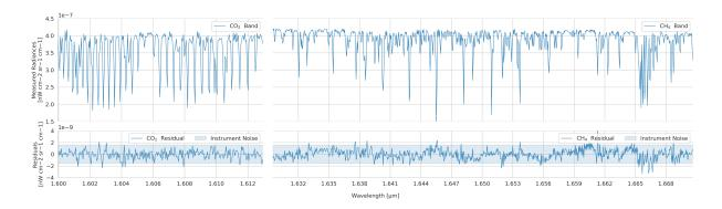
**Figure 2.** Spectra showing the GOSAT radiances for the  $CO_2$  and  $CH_4$  bands and the resulting residuals (measured - simulated spectral differences). The data shown are the median values for the 25,274 land retrievals that pass the quality filtering for an example month, August 2016.
