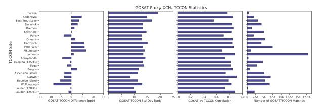
**Figure 6.** Summary of the statistics from Figure 5 comparing the GOSAT Proxy XCH<sub>4</sub> data to the TCCON measurements for each TCCON. Panels show the GOSAT-TCCON difference, the GOSAT-TCCON standard deviation, the correlation coefficients between the GOSAT and TCCON data and finally the number of co-located GOSAT-TCCON measurements.
