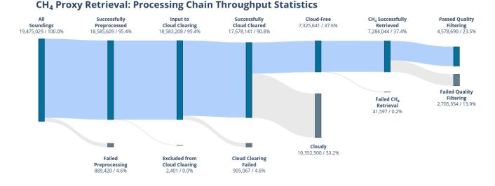
Figure 3. Sankey diagram detailing the retrieval throughput at each step of the processing chain for the GOSAT Proxy XCH<sub>4</sub> retrieval. As well as the absolute number of soundings, the percentage relative to the initial total is also given.
