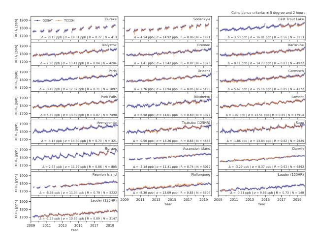
**Figure 5.** Time series plots for each TCCON site comparing GOSAT Proxy XCH<sub>4</sub> data to the matching co-located TCCON measurements. Statistics for each site are included, showing the average GOSAT-TCCON difference, the GOSAT-TCCON standard deviation, the correlation coefficients and the number of co-located GOSAT-TCCON measurements.
