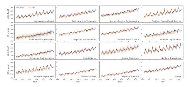
**Figure 12.** Time series comparison between the GOSAT Proxy XCH<sub>4</sub> data and TM5 model XCH<sub>4</sub> simulations (Bergamaschi et al., 2018b) for individual TransCom regions. The model data has been sampled at the time/location of the GOSAT observation and had the sounding-specific GOSAT averaging kernel applied.
