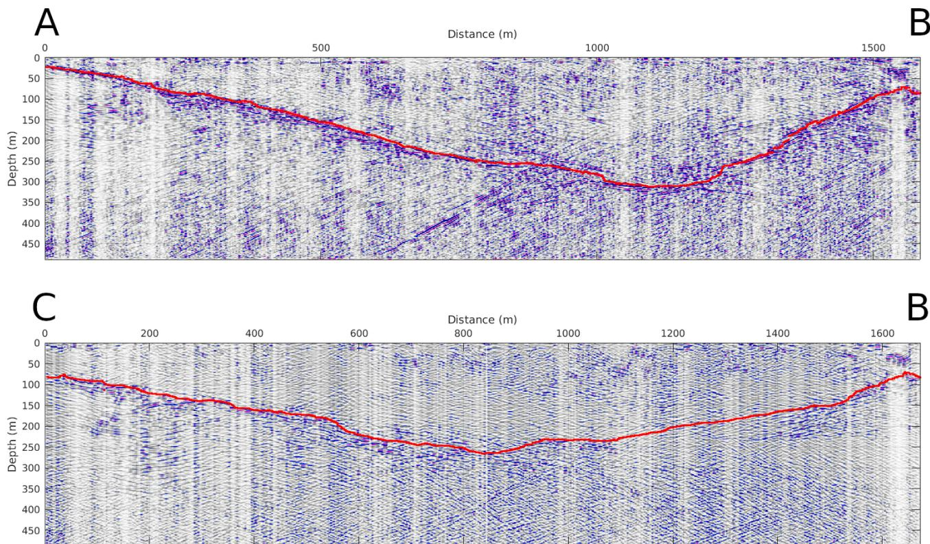
**Figure 3.** Resulting radargrams showing the manually interpreted bedrock in red from Southwest to Northeast. The x-axis shows the distance covered during the measurements. The y-axis represents the estimated bedrock depth in meters.
