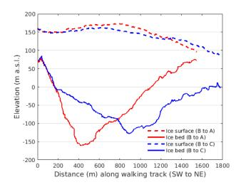
Figure 4. Ice surface and glacier bed elevation along the profiles shown in Figure 2.
