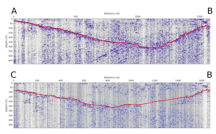
**Figure 3.** Resulting radargrams showing the manually interpreted bedrock in red from Southwest to Northeast. The x-axis shows the distance covered during the measurements. The y-axis represents the estimated bedrock depth in meters.
