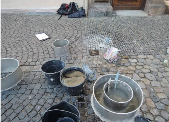
Figure 5: Infiltration experiments at the plots of cluster D
