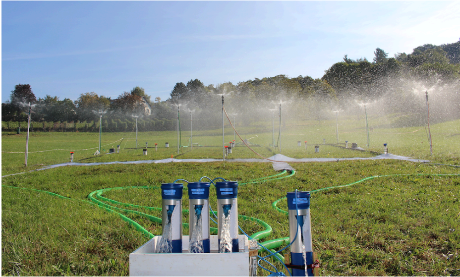
Figure 3: Exemplary setup of the field experiments. The foreground shows the measurement device for surface and subsurface runoff and the connecting lines (green hoses) from the trench covered with plastic sheets. Visible in the background is the actual experimental plot divided into the three subplots with rainfall gauges and the sprinkling system.
