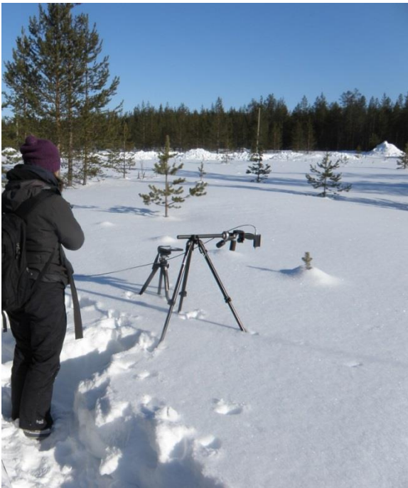
295 Figure 7. Measurement set-up for field measurements with the ASD Field Spec Pro JR spectroradiometer. During the measurement, the operator moved further off and squatted to minimize the effect on the measurements.
