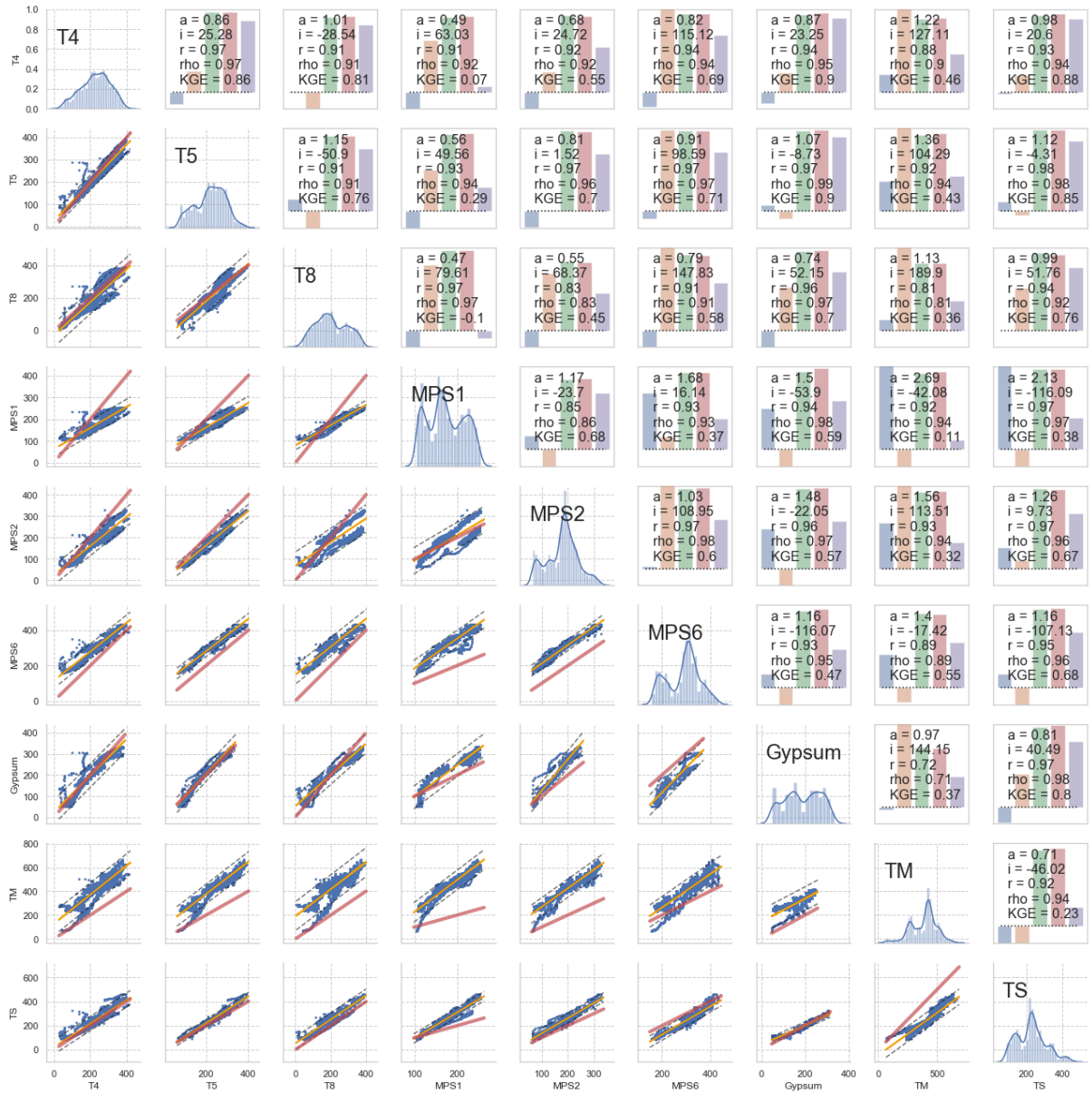
Figure 7. Correlation matrix of all plausible sensor systems for matric potential (given in hPa). Diagonal panels give histogram and kernel density distribution of 0.5 h means of all sensors of one system. Lower half give scatter plot (blue dots), linear regression (orange line), 0.95 predictive uncertainty bands (grey dashed lines), and the 1:1 line (red). The upper half reports the respective correlation measures with a and i as scaling factor and intercept of the linear regression model, r as Pearson correlation coefficient, \rho as Spearman rank correlation coefficient, and KGE as Kling-Gupta-Efficiency. These values are plotted as bars in the same order in the background, where a is plotted as deviation from unity and i is scaled with 0.01.
