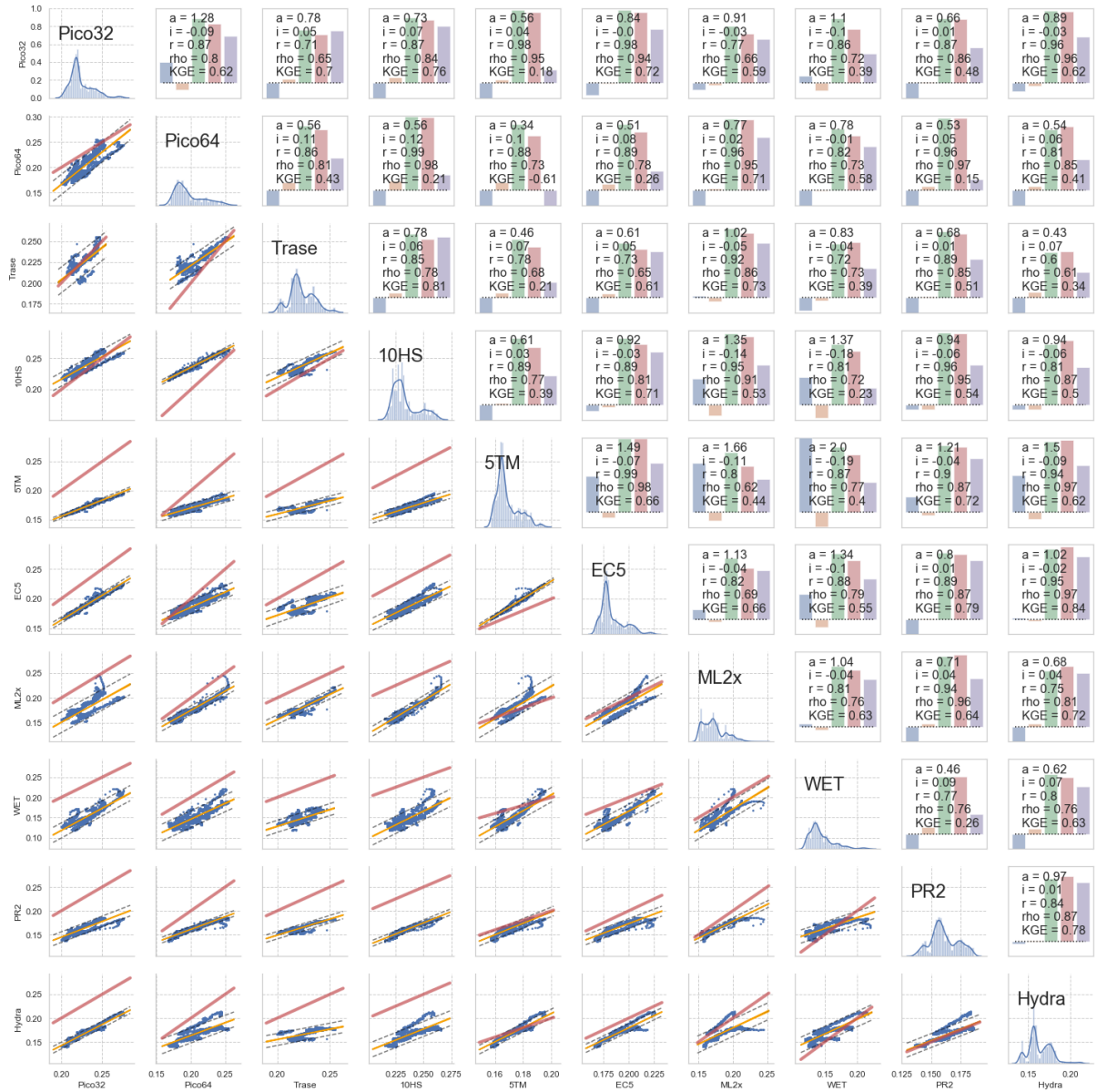
Figure 6. Correlation matrix of all plausible sensor systems measuring soil moisture (given in \text{m}^3/\text{m}^3 ). Diagonal panels give histogram and kernel density distribution of 0.5 h means of all sensors of one system. Lower half give scatter plot (blue dots), linear regression (orange line), 0.95 predictive uncertainty bands (grey dashed lines), and the 1:1 line (red). The upper half reports the respective correlation measures with a and i as scaling factor and intercept of the linear regression model, r as Pearson correlation coefficient, \rho as Spearman rank correlation coefficient, and KGE as Kling-Gupta-Efficiency. These values are plotted as bars in the same order in the background, where a is plotted as deviation from unity.
