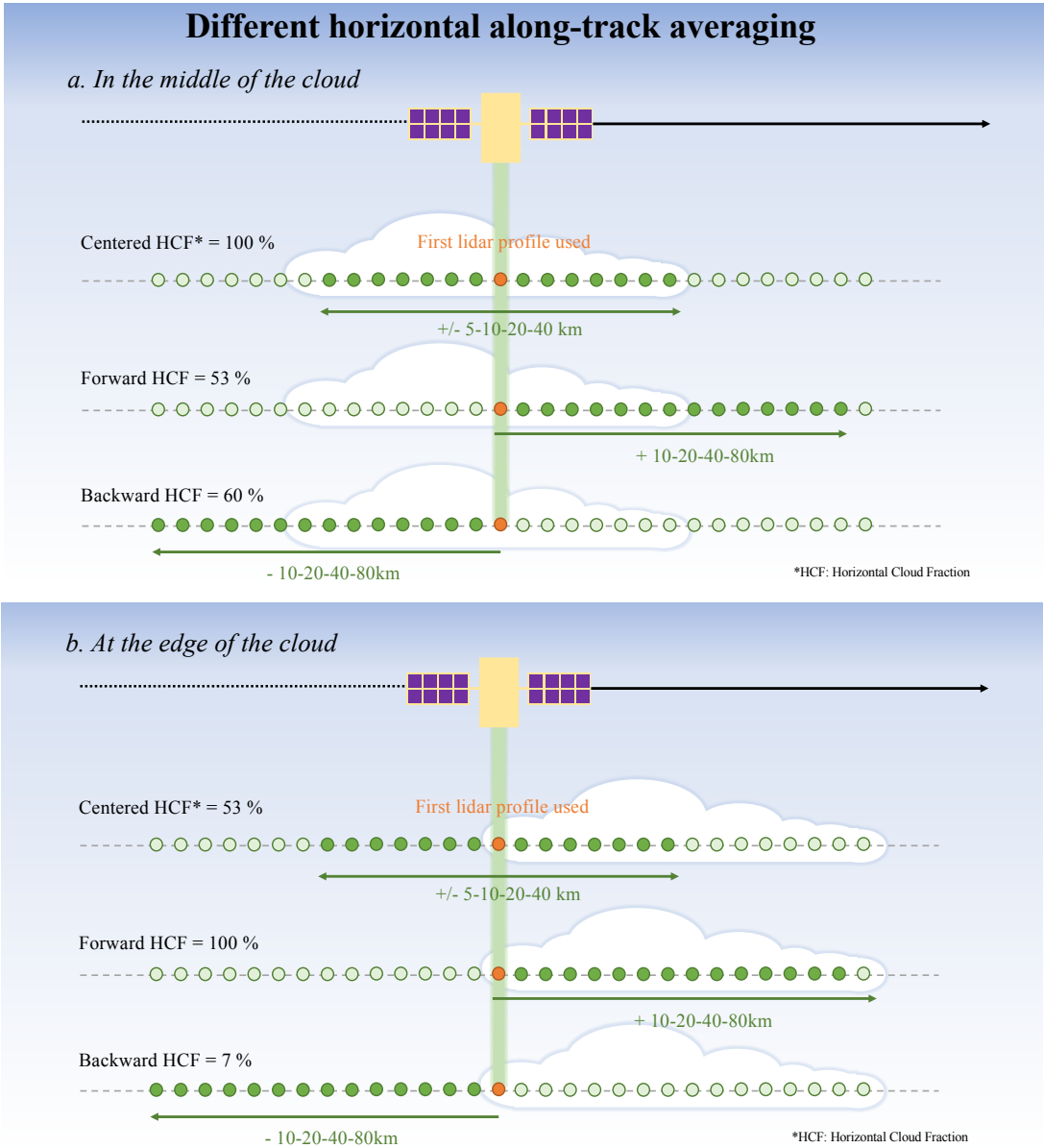
Figure 3: Cartoon of the horizontal along-track averaging that is used by the DA to compute the horizontal cloud fraction (HCF): a) the lidar beam is in the middle of the cloud and b) the lidar beam is at the edge of the cloud. The dark-green circles correspond to the profiles used to in the different horizontal averaging scenarios (centered, forward or backward).
