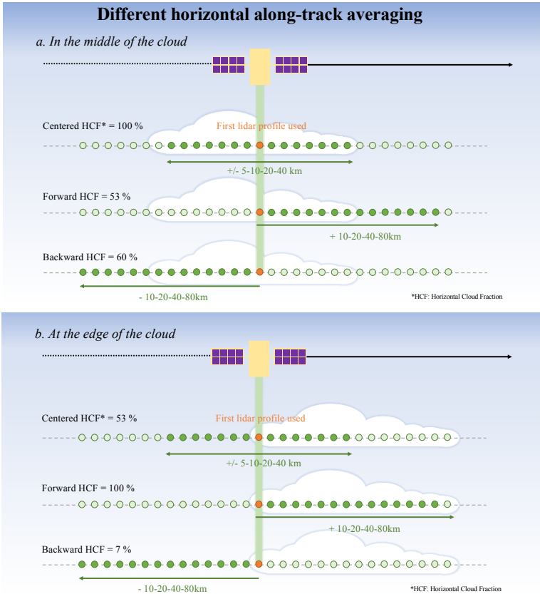
Figure 3: Cartoon of the horizontal along-track averaging that is used by the DA to compute the horizontal cloud fraction (HCF): a) the lidar beam is in the middle of the cloud and b) the lidar beam is at the edge of the cloud. The dark-green circles correspond to the profiles used in the different horizontal averaging scenarios (centered, forward or backward).
