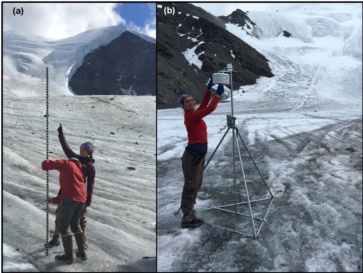
Figure 5. Examples of (a) ablation stakes (lower site) and (b) weather stations (upper site) installed on Chamberlin Glacier.
