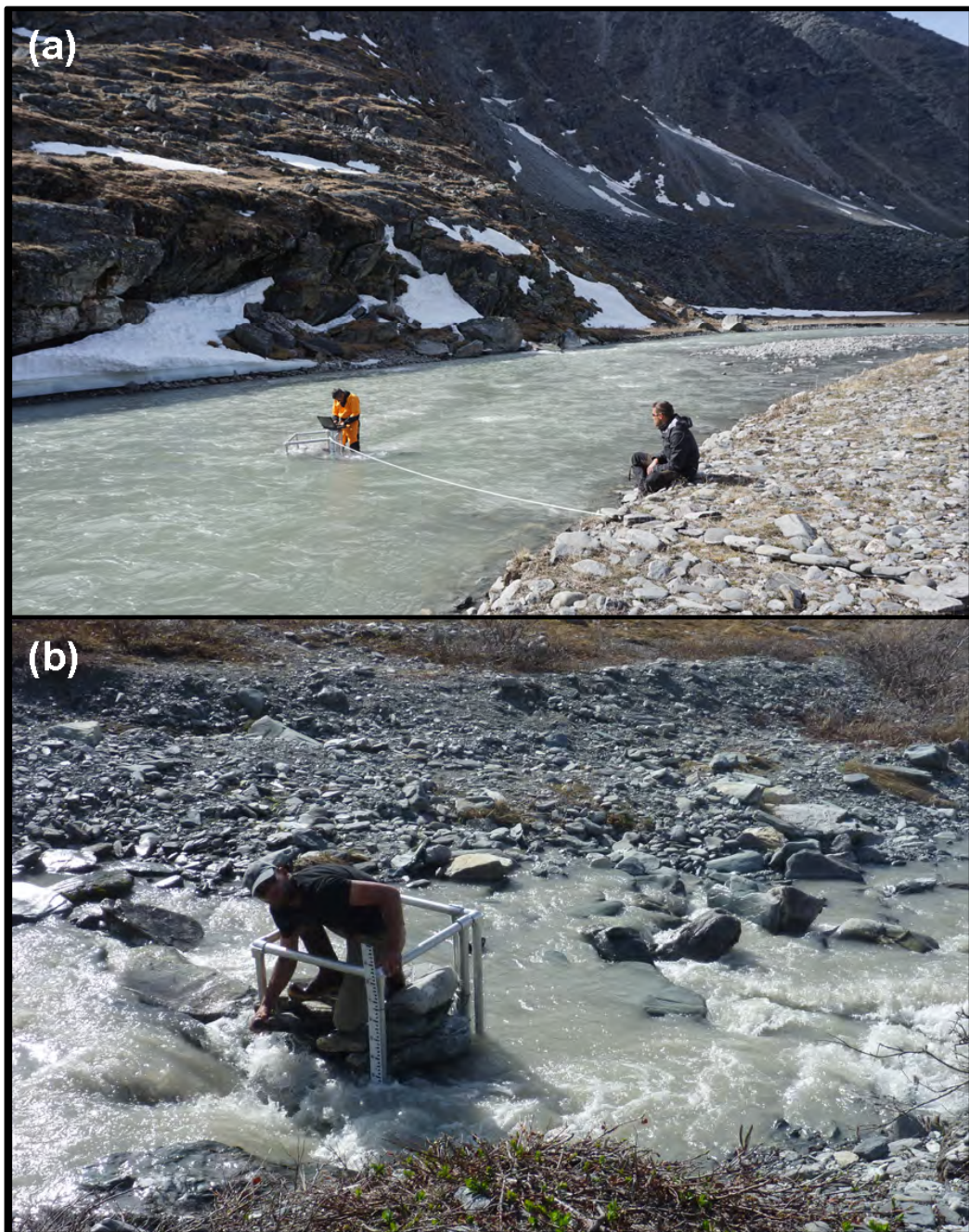
565 Figure 6. Stream stage gauges for (a) Carnivore and (b) Chamberlin Creeks. Instrumentation mounted in tubing is obscured by stage gages.
