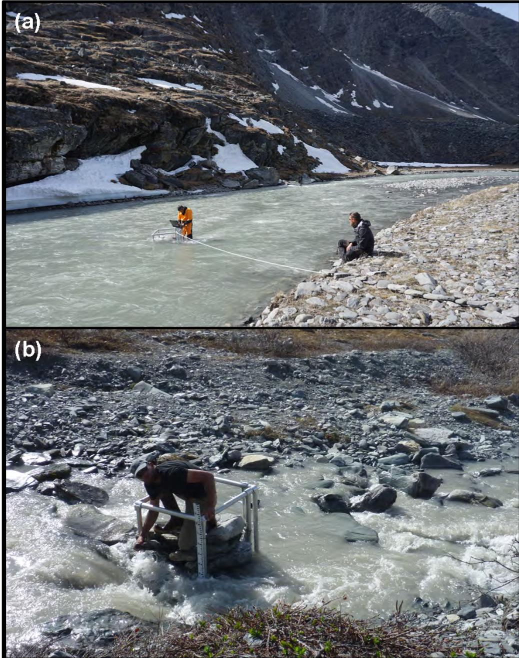
Figure 6. Stream stage gauges for (a) Carnivore and (b) Chamberlin Creeks. Instrumentation mounted in tubing is obscured by stage gages.
