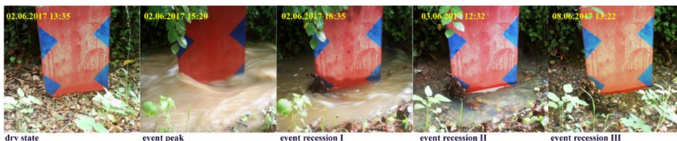
Figure 2: Example of streamflow event classification (site ID: C34) with change from dry to wet state and back. The event starts between 13:35 and 15:20 on the 02.06.2017. Images taken between the time steps of dry conditions and event peak have been automatically identified by the software as being too noisy. Flow decreases during the event recession and ends on the 10.06.2017.
