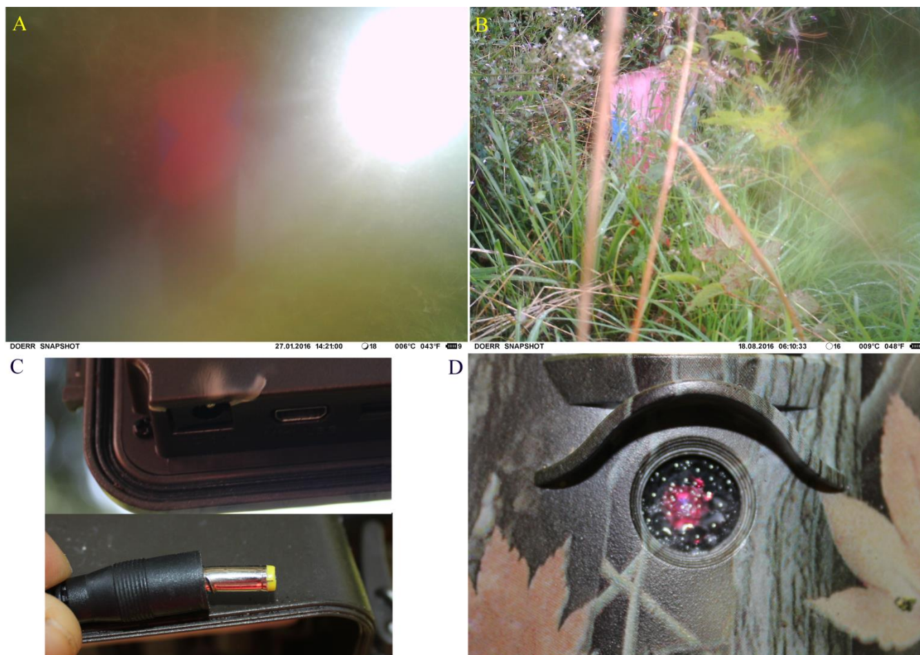
Figure 8: Sources of uncertainties and errors in the time-lapse imagery data. A) reflections of sublight into the lens, B) growth of vegetation between camera and stream, C) damaged cable connection after attempted SD-card theft or D) by condensated water within the lens system.
