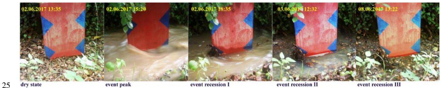
Figure 2: Example of streamflow event classification (site ID: C34) with change from dry to wet state and back. The event starts between 13:35 and 15:20 on the 02.06.2017. Images taken between the time steps of dry conditions and event peak have been automatically identified by the software as being too noisy. Flow decreases during the event recession and ends on the 10.06.2017.
