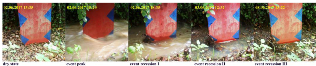
25 Figure 2: Example of streamflow event classification (site ID: C34) with change from dry to wet state and back. The event starts between 13:35 and 15:20 on the 02.06.2017. Images taken between the time steps of dry conditions and event peak have been automatically identified by the software as being too noisy. Flow decreases during the event recession and ends on the 10.06.2017.
