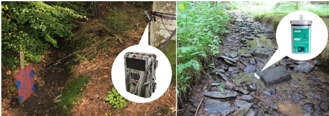
Figure 3: Sensor setup for time lapse camera (left) and EC-sensor (right). The EC-sensor housing is mounted to a concrete block in the streambed.
