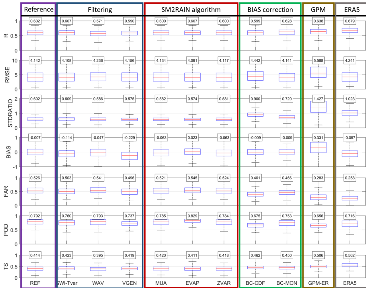
751 Figure 3. Performances at 1009 points in terms of Pearson’s correlation, R [-], root mean square 752 error, RMSE [mm/day], variability ratio, STDRATIO [-], BIAS [mm/day], false alarm ratio, 753 FAR [-], Probability of Detection, POD [-], and Threat Score, TS [-]. For details of the different 754 configurations see Table 2 (GPM-ER: GPM IMERG Early Run product).
