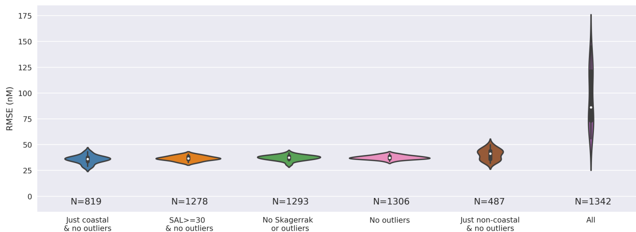
Figure A1. Combined kernel density and boxplots (“violin plots”) showing the distribution of Root Mean Square Error (RMSE) for 20 different models built from 20 different pseudo-random initialisations for different selection of the dataset as described in Table 2 and Sect 3.2. Models built using the whole dataset (“all”), including outliers, show a significantly higher RMSE due to observations with higher iodide concentrations. The model used here includes ancillary variables of temperature, depth and salinity which were thought to intuitively give a reasonable result.
