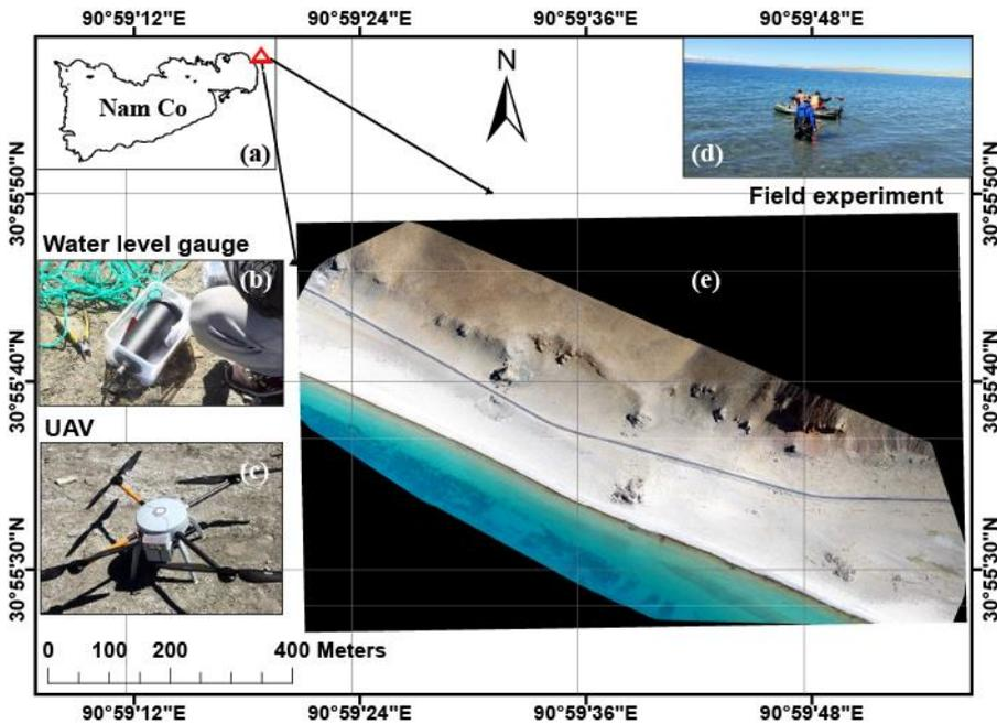
**Figure 7.** Field experiments in two typical study-lakes: (a) an overview map of the experiment spot; (b) pressure-type water level sensor; (c) unmanned aerial vehicle (UAV); (d) installation of the water level sensor; and (e) UAV image of a portion of the bank of Nam Co.
