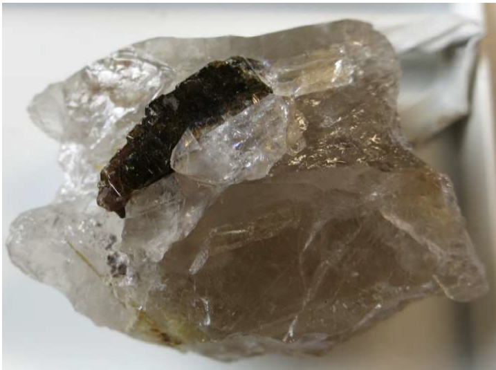
Figure 3: Xenotime embedded in quartz as an example for the REE-bearing mineral samples.
