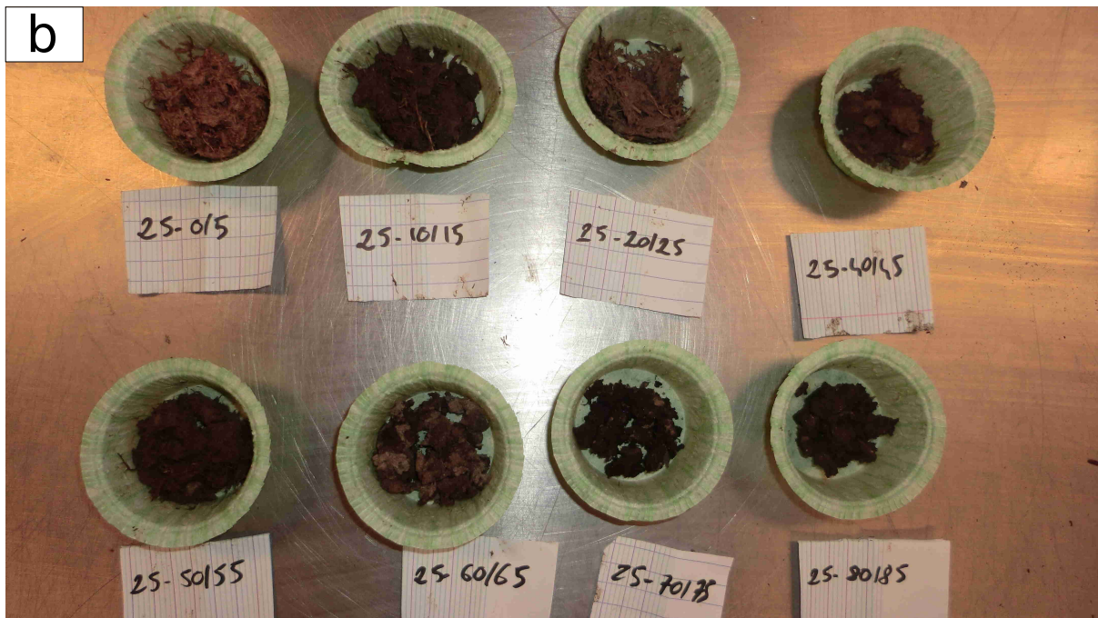
Figure 4. First transect soil samples after 48 hours of oven drying at 80 °C. Different samples depths are shown for plots (a) : T1 – 10 ; (b) : T1 – 25.
