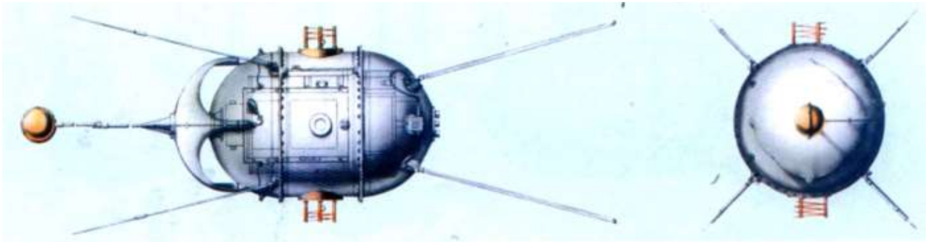
Figure 1: External view of the DS-MG type spacecraft (Kosmos-26 and Kosmos-49), 1964 (Konyukhov, 2000).
