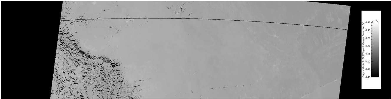
Figure 1. Example of missing lines (in this case two consecutive lines) in the L1B2 terrain-projected LOCAL MODE bidirectional reflectance factor data for the blue spectral band of the DF camera for PATH 168, ORBIT 68 050 and BLOCK 110, covering an area located in eastern South Africa. The linear gray scale, shown on the right side of the frame, assigns Brf values of 0 to black and Brf values of 0.35 or higher to white. The black spots on the western side of the map are due to pixels that are not observed at this slanted view angle due to the local topography. North is approximately towards the top of the image. The total size of the BLOCK area is 563.2 km across-track (roughly west–east) by 140.8 km along-track (roughly north–south), while the parallelogram-shaped ground area inside the BLOCK is about 380 km across-track.
