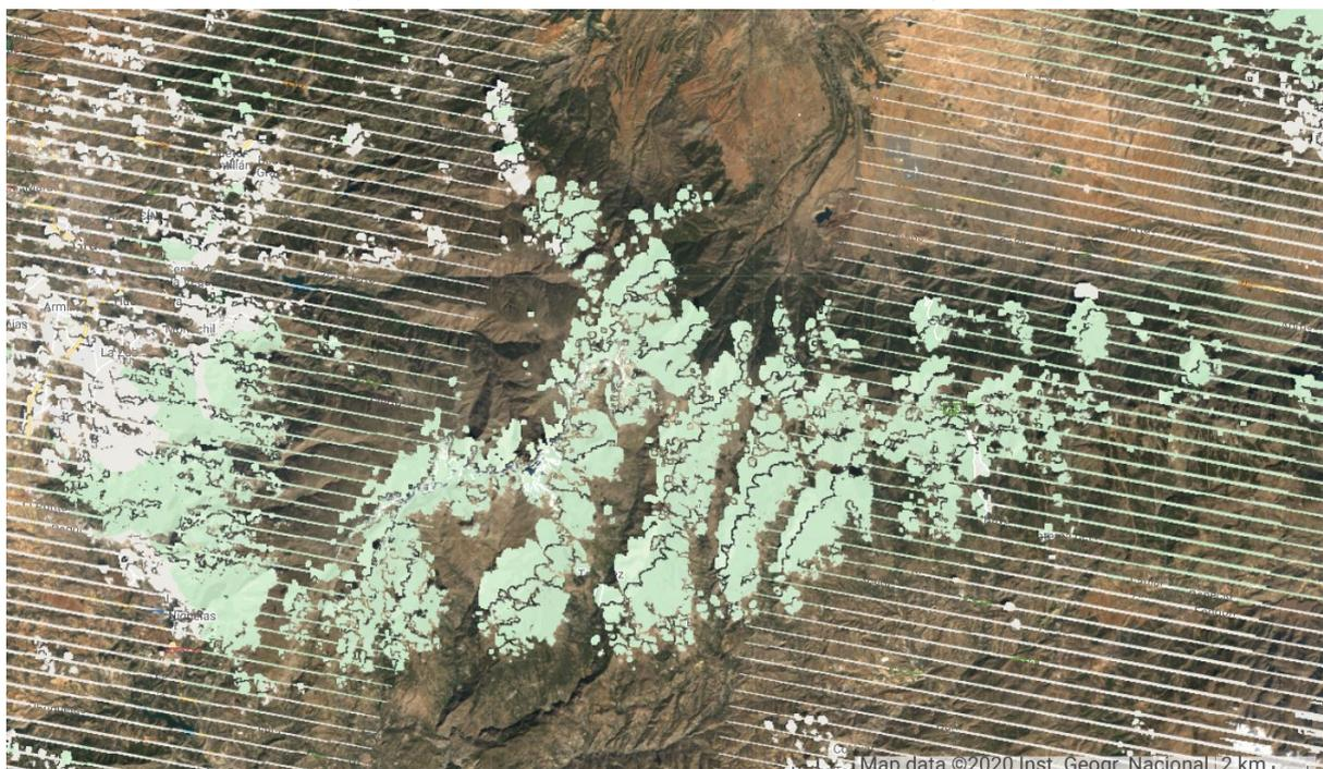
Figure 4. Effect of Scan Line Corrector fault on Landsat7 imagery in Sierra Nevada and data gaps due to clouds (in green and white). Landsat-7 image courtesy of the U.S. Geological Survey.
