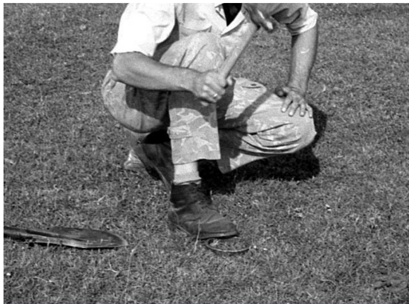
532 533 534 Figure 2. Soil sampling using a ring of 14 cm diameter to collect a 5 cm deep soil core (courtesy 535 of UIAR, 1989).
