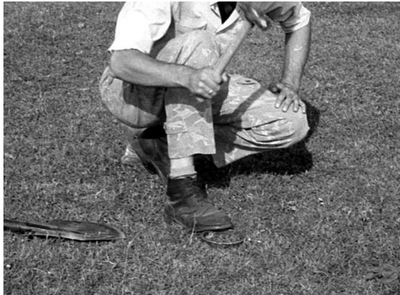
531 532 533 Figure 2. Soil sampling using a ring of 14 cm diameter to collect a 5 cm deep soil core (courtesy 534 of UIAR, 1989).
