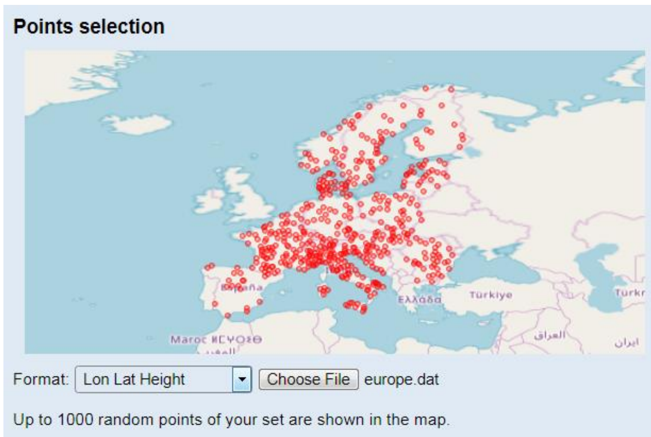
Figure 13: Snapshot of the point value calculation service on ICGEM. The example shows the GNSS/levelling benchmark points in Europe that are used also in the ICGEM static model evaluation. The user can choose one, multiple or all the functionals at the same time to compute at those points.
