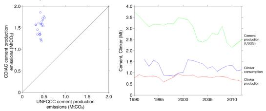
Figure A3: Netherlands. Left: CDIAC vs UNFCCC. Right: Clinker, cement. Note 'Clinker consumption' is production plus imports less exports, but excludes stock changes. Sources: (van Oss, 1994–2019; Boden et al., 2013; UNFCCC, 2014; UNSD, 2015).
