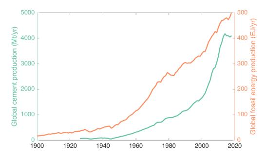
Figure 1: Global cement and fossil energy production to 2018 (Mohr et al., 2015; USGS, 2016, 2018; BP, 2019).
