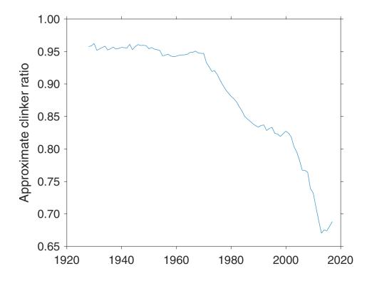
Figure A1: Approximate implied global clinker ratio, derived from emissions estimates and cement production data using default emission factors. The trend up until 1990 is largely a result of the assumptions used in extrapolation, although in earlier years the data for the US and Europe dominate.
