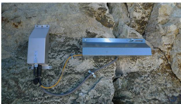
**Figure D5.** Close up of crackmeter and thermistor chain installation at position MH03. The wireless sensor node is housed in the steel protective shoe on the left while the crackmeter is located under the steel protective shield in the middle.
