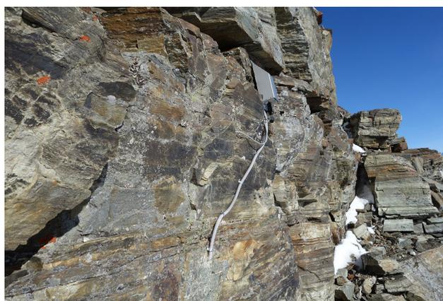
**Figure D7.** Rock temperature measurement at position MH10 on a south exposed rock face.
