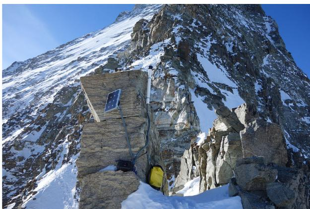
**Figure D10.** Wireless L1-GPS installed at position MH34 monitoring the gradual tilting of a little tower feature that is separated from the main ridge.
