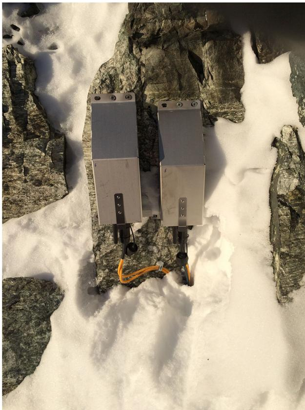
**Figure D9.** Sensor nodes at position MH05 and MH06 are installed on a small rock wall above a ledge to prevent heavy snow coverage while the sensors themselves are not visible.
