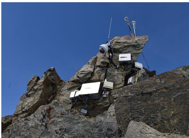
**Figure D4.** A Vaisala WXT520 weather station and Kipp & Zonen CNR4 radiometer are installed on top of the ridge crest. Other equipment shown here are a webcam, Leica GRX1200+ high-precision GNSS receiver and the required wireless transmission and power control equipment.
