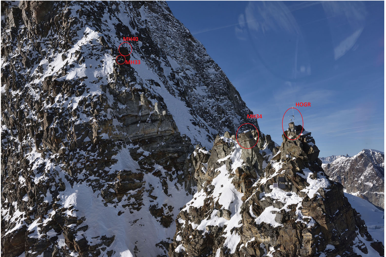
Figure C12. Closeup of the detachment zone (middle) and the butte between first and second couloir. The instrument cluster around and below GNSS measurement position MH42 / HOGR (right) contains the weather station, webcam, high-resolution camera and sensor network base station.
