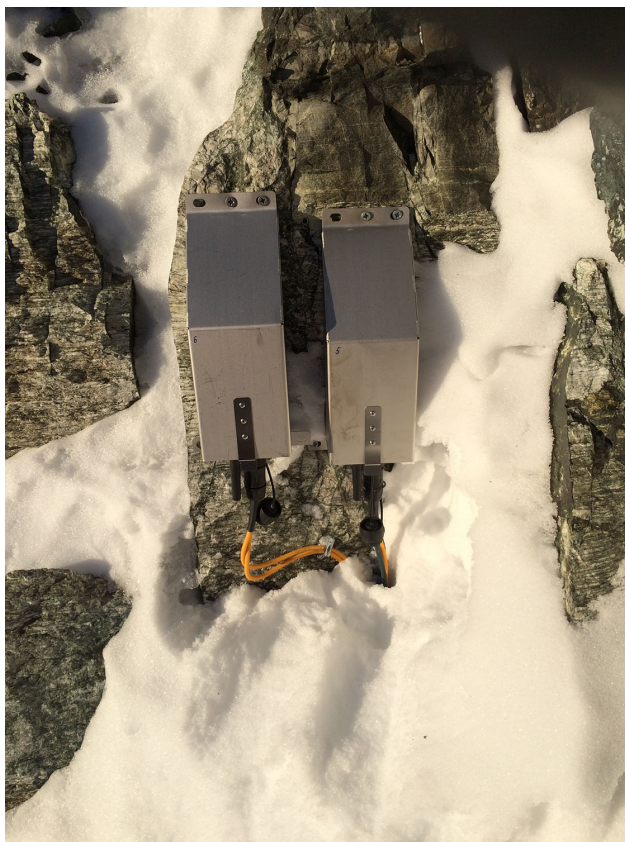
Figure C9. Sensor nodes at position MH05 and MH06 are installed on a small rock wall above a ledge to prevent heavy snow coverage while the sensors themselves are not visible.
