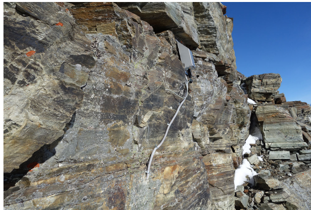
Figure C7. Rock temperature measurement at position MH10 on a south exposed rock face.
