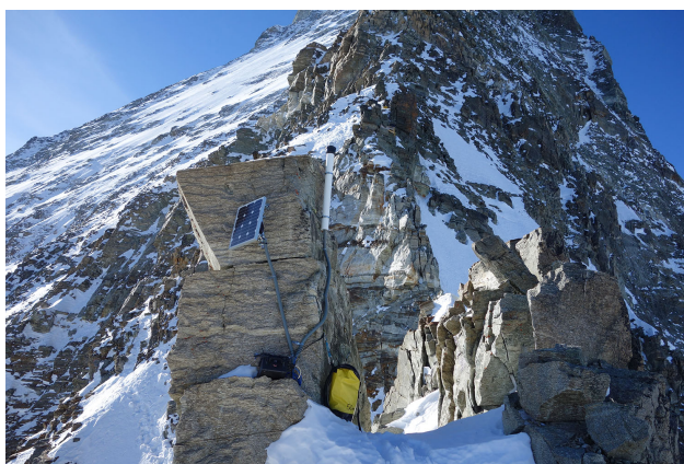
Figure C10. Wireless L1-GPS installed at position MH34 monitoring the gradual tilting of a little tower feature that is separated from the main ridge.
