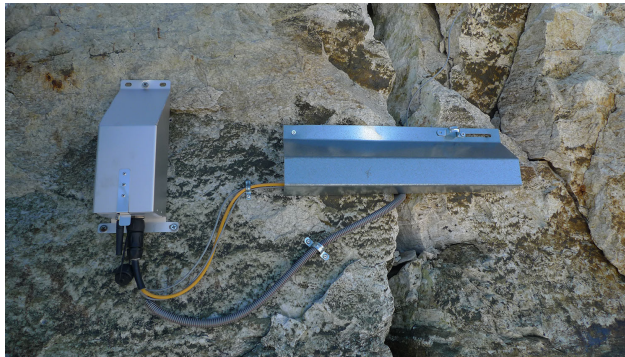
Figure C5. Close up of crackmeter and thermistor chain installation at position MH03. The wireless sensor node is housed in the steel protective shoe on the left while the crackmeter is located under the steel protective shield in the middle.
