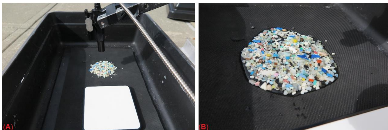
Figure 1 Experimental setup with the aggregated (A) dry and (B) wet marine harvested microplastics. A black neoprene rubber was used as a background in a dark spray painted container to mitigate background light during spectral reflectance measurements.
