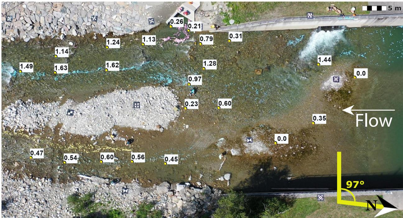
**Figure 3.** A snapshot from the footage collected near a fish ladder and distribution of reference measurements with corresponding velocity magnitudes ( $\text{m s}^{-1}$ ). The dominant direction of flow is indicated by the arrow.
