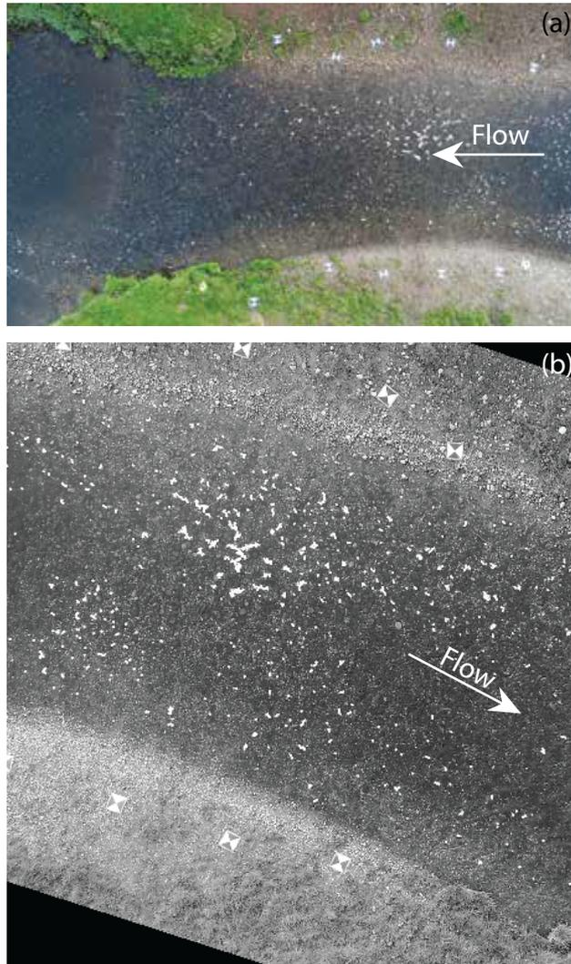
**Figure 2.** (a) Footage acquired by the Phantom 4 UAS over the River Arrow, and (b) following orthorectification and grayscale conversion. The Ecofoam chips and ground control points are clearly visible in both images. The direction of flow is indicated by the arrows.
