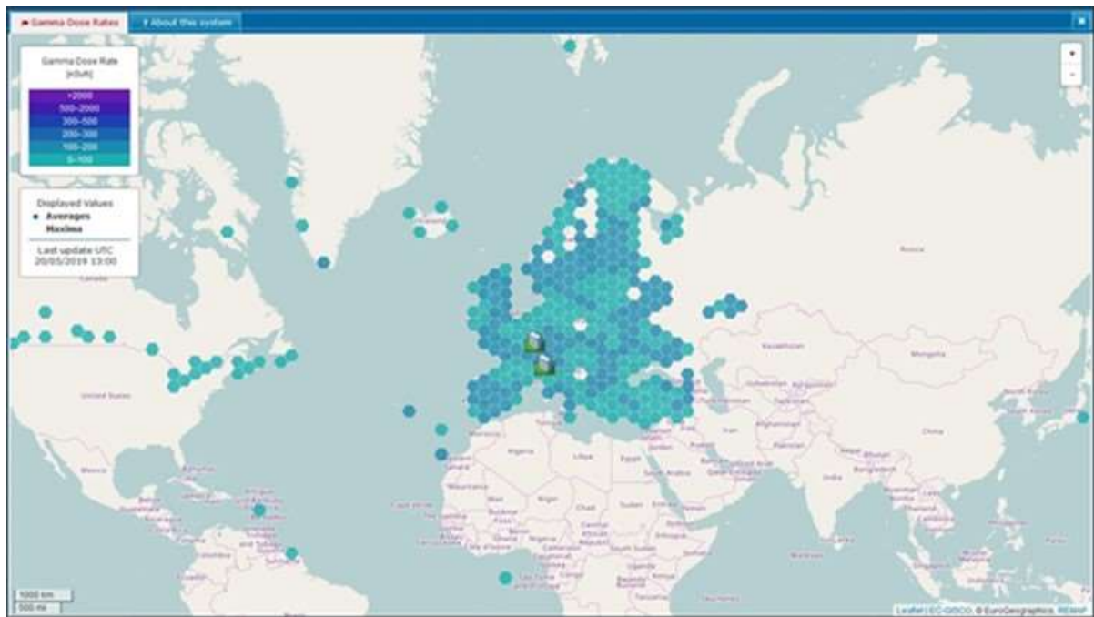
Figure 3. Screenshot of the EURDEP Public Map. This map shows the maximum and the average value of total gamma dose rate for each hexagon considering the stations inside, which have reported measurements during the last 24 hours and considering values as time-averaged values. (Developed by EC JRC)
