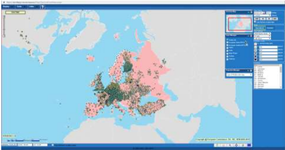
Figure 2. Screenshot of the EURDEP “expert map” showing the locations of the gamma dose rate monitoring stations. (Copyright © European Commission. DG. JRC, REM 2009-2019)
