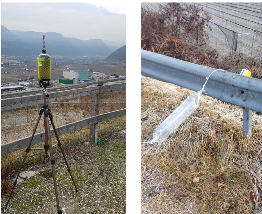
Figure 2. Vacuum-filled glass bottle (left) and PVF bag (right) used to collect samples of ambient air. These pictures were taken during the tracer releases of BTEX. On the right of the vacuum bottle, the incinerator of Bolzano can be recognised.
