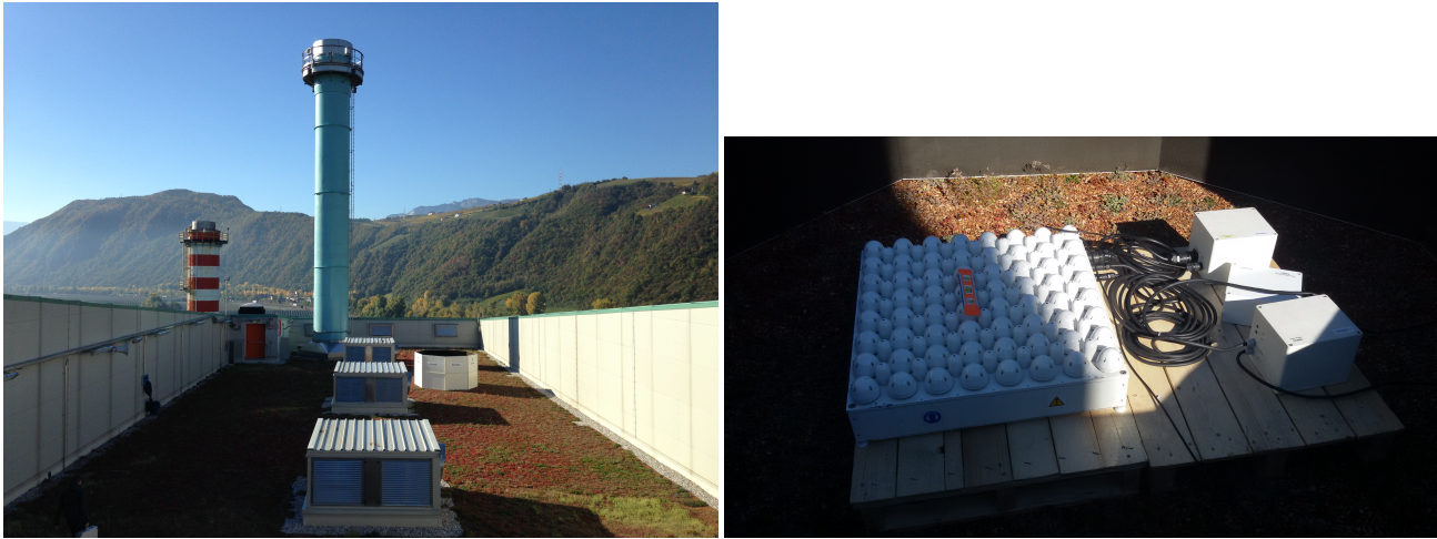
Figure 3. A view on the roof of the incinerator of Bolzano during the experimental campaign with the MFAS mini-SODAR (left) and the detail of the antenna (right).
