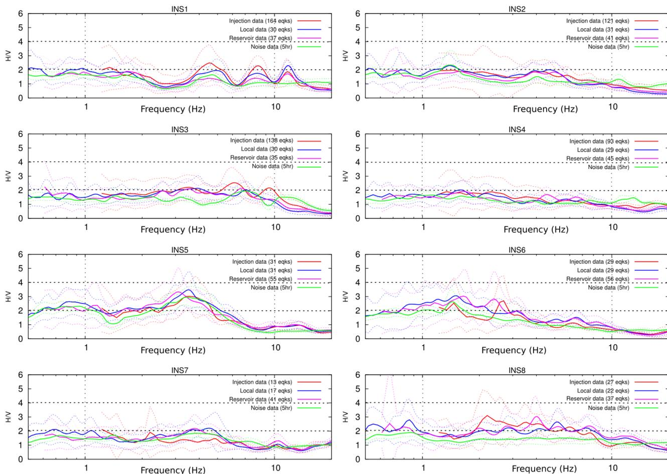
**Figure 8:** HVSR and HVNSR curves computed at all the INSIEME network seismic stations. For each dataset, the number of used earthquakes and the hours of seismic noise are indicated. The solid coloured line represent the average HVSR and HVNSR curves, whereas the dashed lines identify the  $\pm 1\sigma$  standard deviations.
