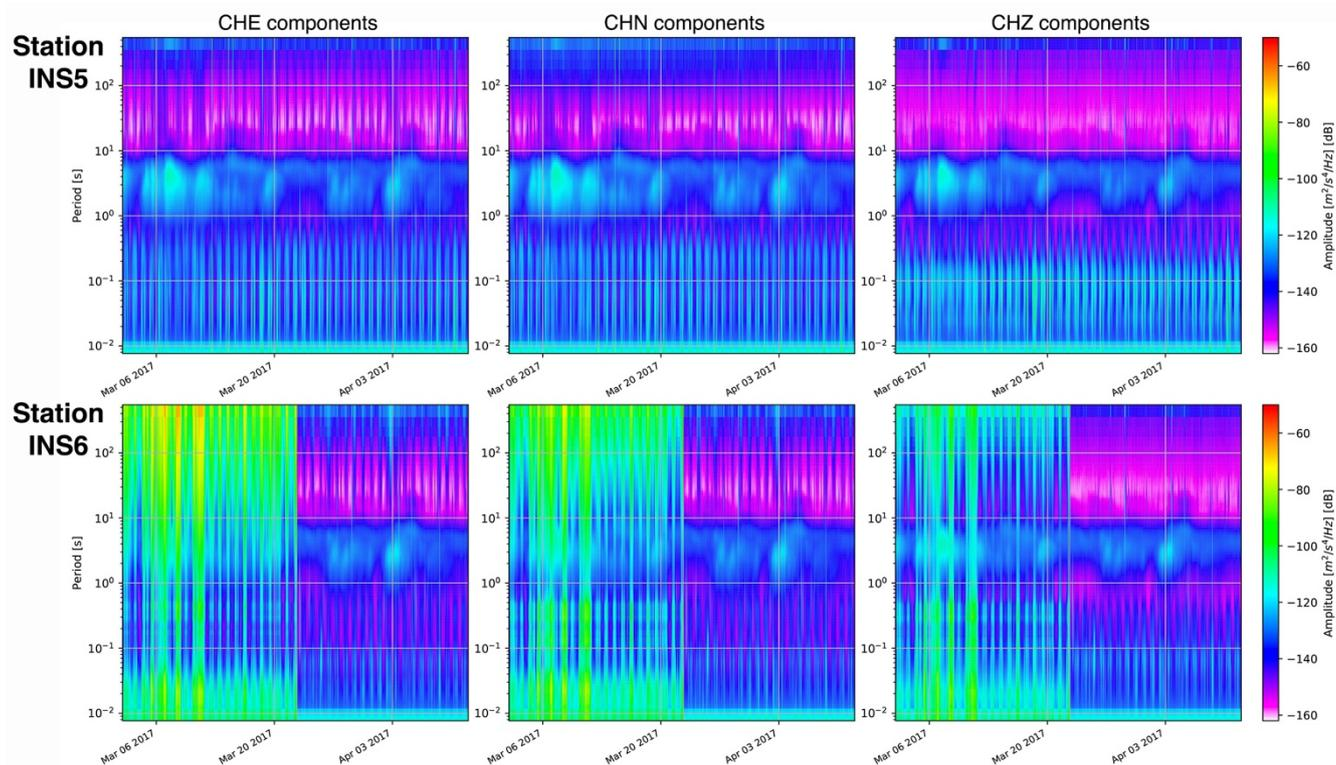
**Figure 7:** Spectrograms of each component of station INS5 (top panels) and INS6 (bottom panels) computed over continuous data streams of 41 days (from 2017-03-02 to 2017-04-11). The sensor of station INS5 was installed at 6 m depth for the whole period of observation whereas the sensor of station INS6 was first installed on surface and then moved at 6 m depth on 2017-03-22.
