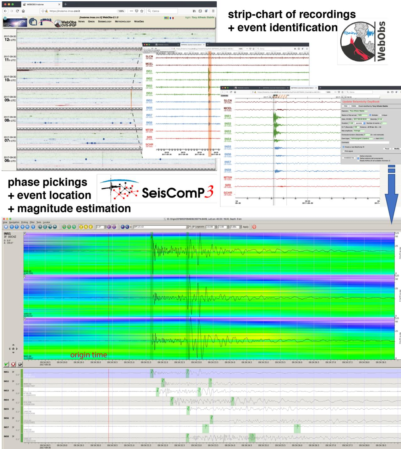
Figure 4: Tools implemented for visualization and processing of acquired seismic data. The WebObs intranet system (top panels) is used to plot in near real-time strip-chart of recordings at configured stations any event present in the data. When an event is identified, the information is sent to the SeisComP3 database for the manual phase picking and event location (bottom panel) through the Origin Locator Viewer tool (scolv).
