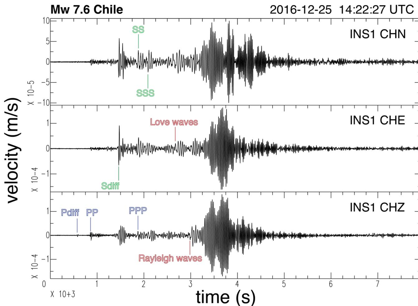
Figure 11: Mw=7.6 Chile earthquake of 2016-12-25 recorded by the three components of the INS1 seismic station. On the top right of the figure the origin time of the teleseism is reported. The theoretical arrival times of the most important recorded seismic phases are shown. The original horizontal components were rotated counter-clockwise by an angle of  $307.8^\circ$  with respect to the North, according to the computations described in detail in section 2.2.
