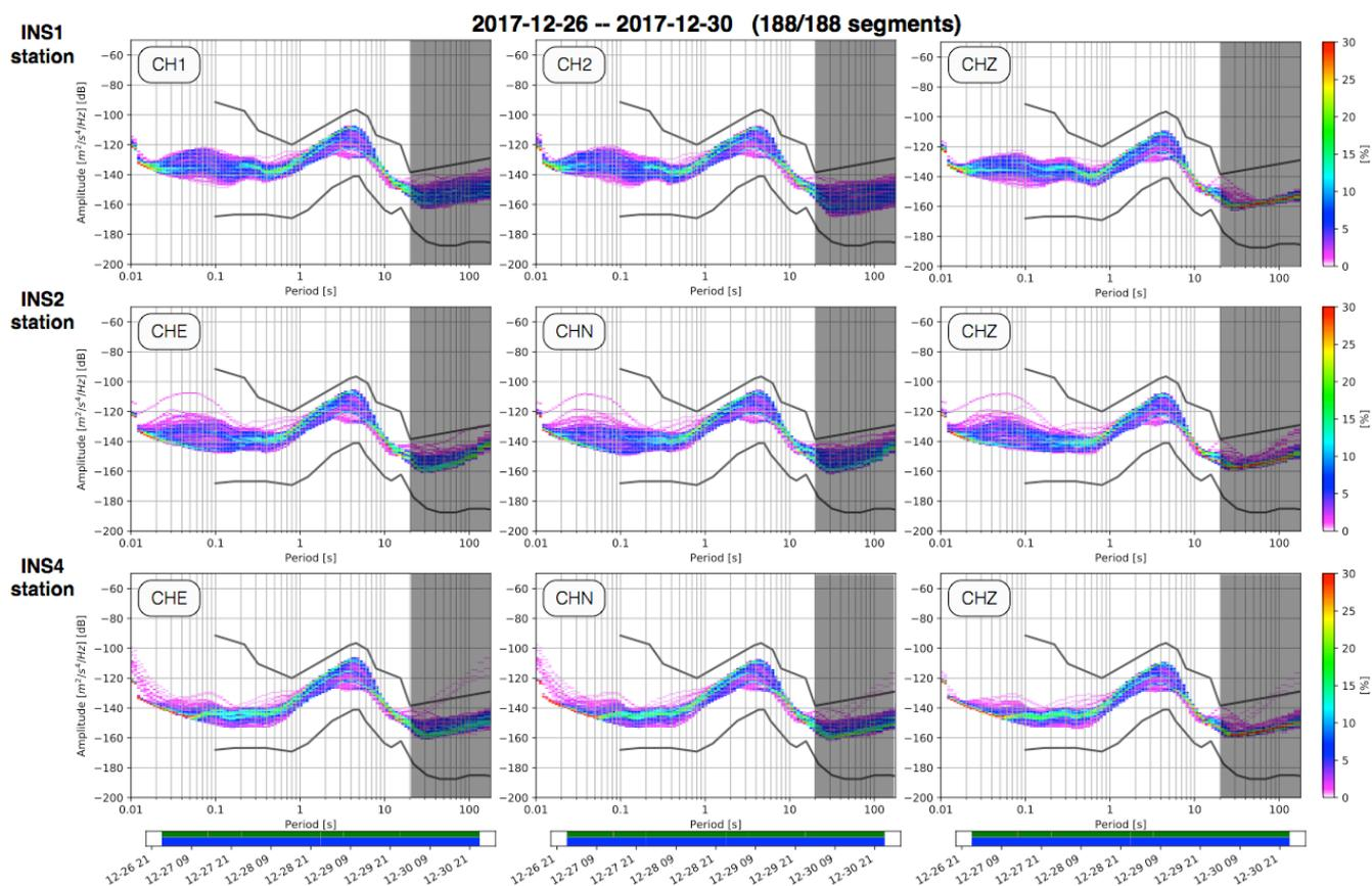
**Figure 6:** Same type of comparison as Figure 5 but among stations INS1 (sensor installed at 50 m depth), INS2 and INS4 (respective sensors both installed at 6 m depth).
