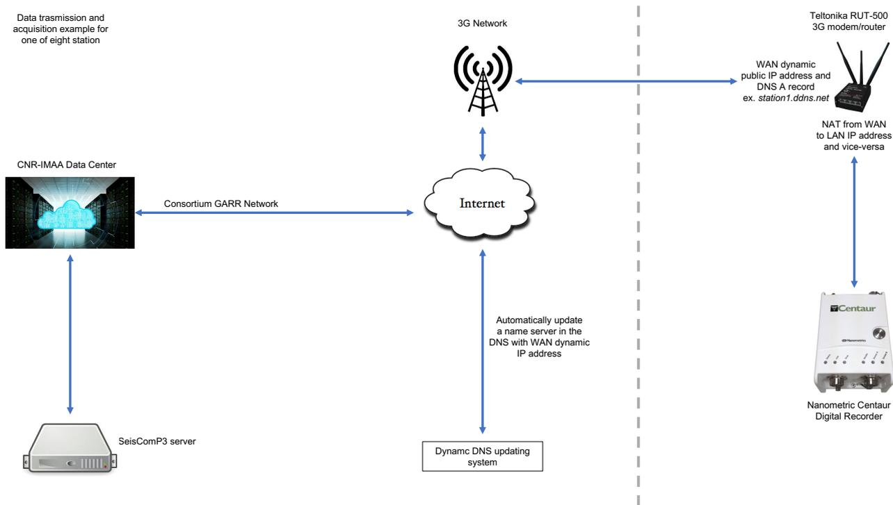
**Figure 3: Schematic view of the data flow from the data-logger of a remote station to the CNR-IMAA Data Centre.**
