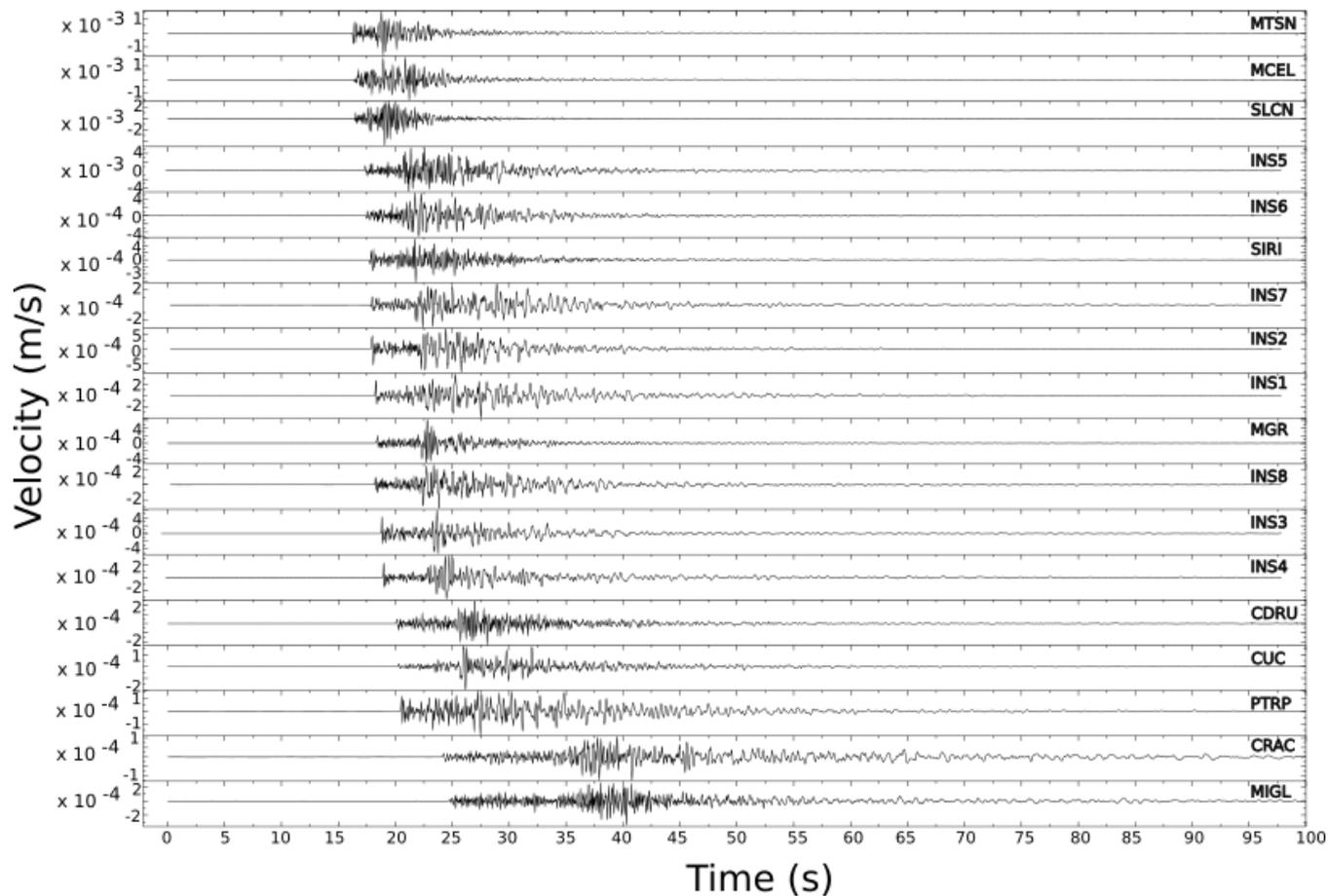
Figure 10:  $M_w=3.8$  local earthquake recorded by the vertical components of the stations belonging to the virtual seismic network composed by INSIEME, INGV and ISNet seismic stations. The traces are sorted, from to the top to the bottom, based on the first P-wave arrival time.
