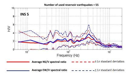
**Fig. 2.** Average HVSR curves retrieved by analyzing the recordings at station INS5 of the reservoir induced events: red and blue lines indicate the HVSR obtained for the NS and the EW component, respectively.
