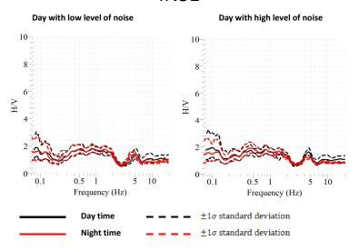
**Fig. 1.** HVNSR curves obtained for INS1 station by using data characterized by low level of noise (left panel) and high level of noise (right panel).
