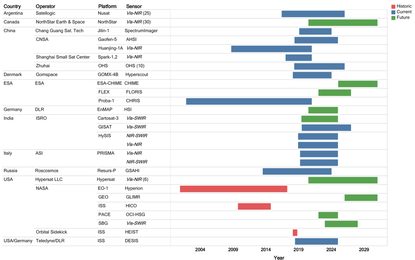
Figure 1. The chart depicts the timeline of historic, existing, and planned high spectral resolution remote-sensing missions by country or agency, operator, platform, and sensor name or type (general sensor type is conveyed in italics). Note that where there is a constellation or multiple sensors for the mission, the number of sensors is given in parentheses at the end of the sensor column.
