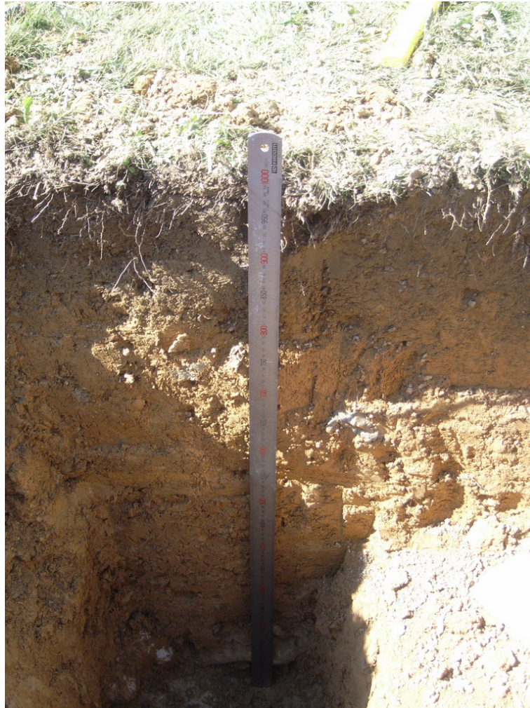
Figure 4. Soil profile of 1 meter depth performed close to location 33 -location 33 on 29 September 2008. The visual characterization provided in Table 1 can be seen on this picture.
