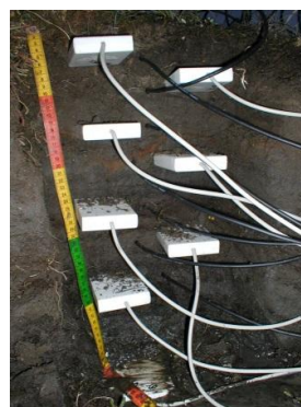
Figure B11. Soil volumetric liquid water content sensors: 20 Campbell Scientific CS605 TDR probes, which are connected to a Campbell Scientific TDR100 time-domain reflectometer, installed on 24 August 2002.
