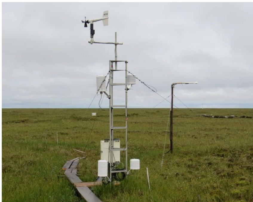
Figure B1. Samoylov meteorological station setup, August 2002–present (72.37001° N, 126.48106° E). Photo taken in August 2015. The two long radiation shields (left side of tower) at heights of 0.5 m and 2 m house the combined temperature and relative humidity probes (two Vaisala HMP155A sensors were installed on 17 September 2017) and the two shorter shields (right side of tower) at the same heights contain Campbell Scientific PT100 sensors (installed on 22 August 2013) to measure air temperature only. The data logger (Campbell Scientific CR1000, installed on 30 June 2009), multiplexer (Campbell Scientific AM16/32A, installed on 27 July 2010) and barometric pressure sensor (Vaisala PTP110, installed on 22 August 2014) are located in the white box at the back of the tower. The wind monitor and radiation sensor are shown in the figures below (Figures B2 and B3).
