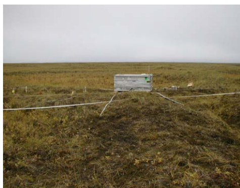
Figure B10. Research site after instrument installation in soil pits and subsequent refilling, August 2002. Cable strings indicate locations of center, slope, and rim profiles.
