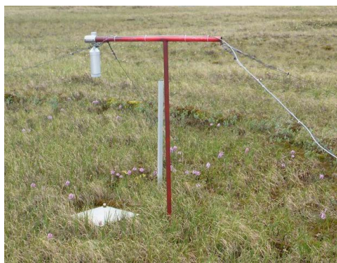
Figure B4. Campbell Scientific SR50 snow depth sensor, installed on 24 August 2002. An aluminum plate was installed on the ground surface beneath the sensor beam on 17 July 2016.
