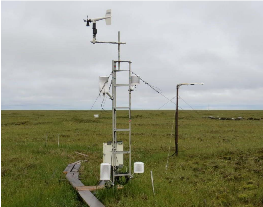
600 Figure B1. Samoylov meteorological station setup, August 2002–present (72.37001° N, 126.48106° E). Photo taken in August 2015. The two long radiation shields (left side of tower) at heights of 0.5 m and 2 m house the combined temperature and relative humidity probes (two Vaisala HMP155A sensors were installed on 17 September 2017) and the two shorter shields (right side of tower) at the same heights contain Campbell Scientific PT100 sensors (installed 605 on 22 August 2013) to measure air temperature only. The data logger (Campbell Scientific CR1000, installed on 30 June 2009), multiplexer (Campbell Scientific AM16/32A, installed on 27 July 2010) and barometric pressure sensor (Vaisala PTP110, installed on 22 August 2014) are located in the white box at the back of the tower. The wind monitor and radiation sensor are shown in the figures below (Figures B2 and B3).
