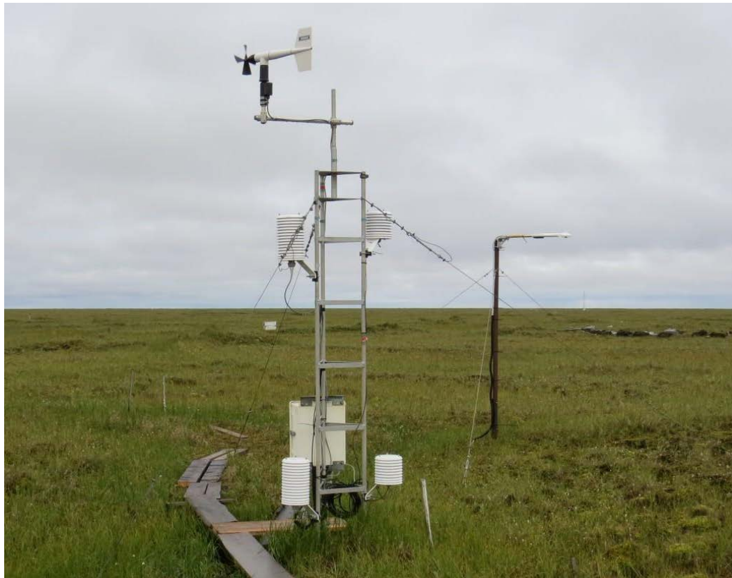
615 Figure B1. Samoylov meteorological station setup, August 2002–present (72.37001° N, 126.48106° E). Photo taken in August 2015. The two long radiation shields (left side of tower) at heights of 0.5 m and 2 m house the combined temperature and relative humidity probes (two Vaisala HMP155A sensors were installed on 17 September 2017) and the two shorter shields (right side of tower) at the same heights contain Campbell Scientific PT100 sensors (installed 620 on 22 August 2013) to measure air temperature only. The data logger (Campbell Scientific CR1000, installed on 30 June 2009), multiplexer (Campbell Scientific AM16/32A, installed on 27 July 2010) and barometric pressure sensor (Vaisala PTP110, installed on 22 August 2014) are located in the white box at the back of the tower. The wind monitor and radiation sensor are shown in the figures below (Figures B2 and B3).
