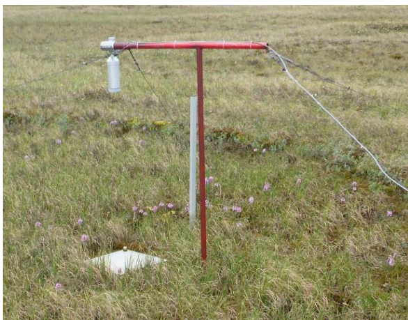
Figure B4. Campbell Scientific SR50 snow depth sensor, installed on 24 August 2002. An aluminum plate was installed on the ground surface beneath the sensor beam on 17 July 2015.
