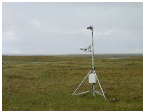
Figure B5. Cameras for time lapse photography of snow cover and land surface pointing towards the polygon field: a Campbell Scientific CC5MPX at the top (since 4 August 2015) and a Campbell Scientific CC640 below (since 1 September 2006). Photo taken in 2016.
