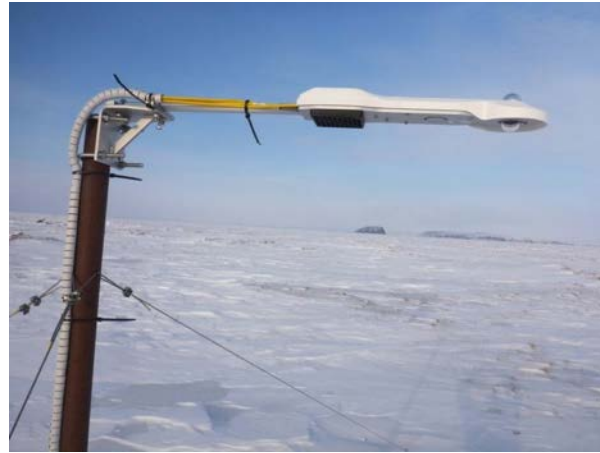
Figure B3. Kipp & Zonen CNR4 radiation sensor (including CNF4 ventilation unit) for measuring incoming and outgoing shortwave and longwave radiation, respectively, installed on 22 August 2014.
