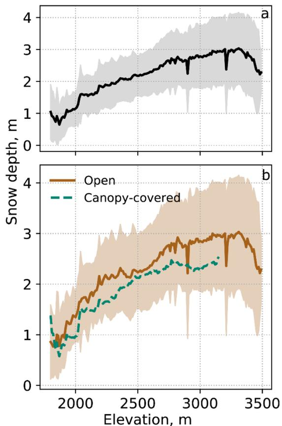
**Figure 1: Snow-depth changes over elevation observed from the lidar data in the Wolverton basin (a) for all snow-depth pixels (b) for snow-depth pixels in the open area and under canopy. On average, snow depth increases with elevation nonlinearly with elevation below 3300 m, decreases when elevation is above 3300 m.**
