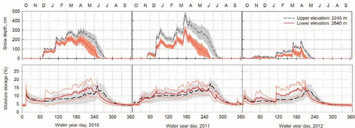
**Figure 4.** The 24 sensor nodes highlight the spatial variability of soil moisture and snow depth through Water Years 2010 (average), 2011 (record-setting wet year) and 2012 (extremely dry). Soil moisture can be higher at the lower elevation than the higher elevation, and peak soil moisture may predate the end of snowmelt.
