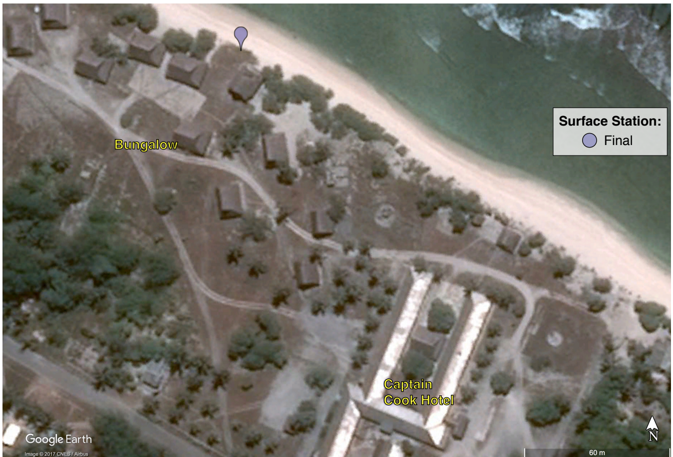
Figure 2: Aerial view of the Captain Cook Hotel property on Kiritimati Island, including the CXENRR site (upper left). The final location of the surface meteorology instruments is at the base of the pin symbol, north-northeast of the bungalow that housed staff and the Vaisala DigiCORA sounding system. The concrete pad where the helium tanks were stored and from which balloons were launched runs northwest to southeast, ending just north of the bungalow. The main hotel building used for internet access is southeast of the CXENRR site.
