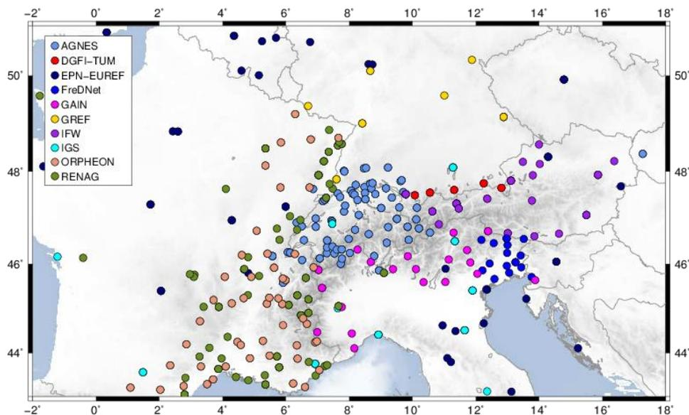
5 **Figure 2: CO-GNSS stations processed for the estimation of the surface-kinematics in the Alps.** The stations of the contributing CO-GNSS arrays are color-coded. Topography and bathymetry after the ETOPO1 model (Amante and Eakins, 2009).
