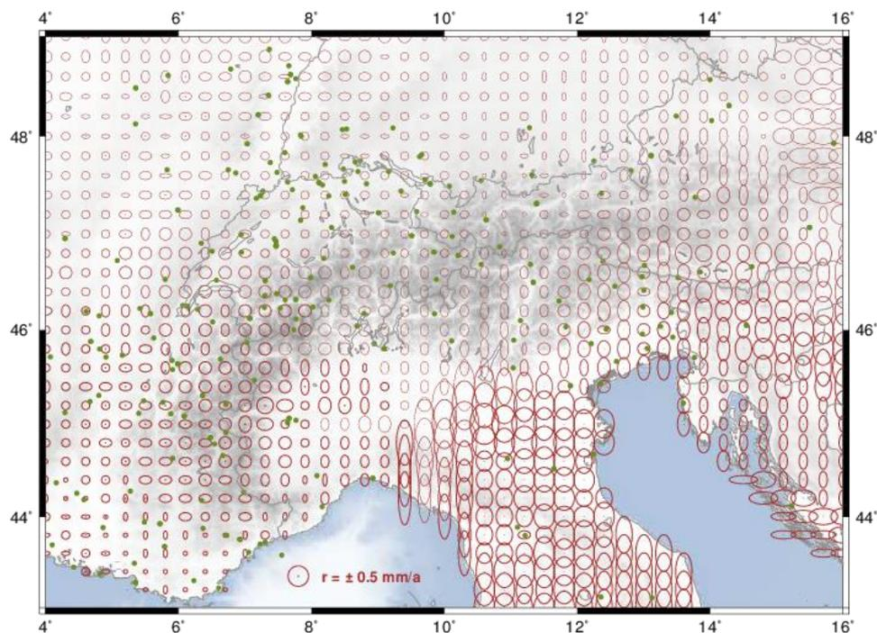
**Figure 10:** Estimated uncertainty (95% confidence) of the GNSS-based horizontal deformation model of the Alpine region. Green dots show the CO-GNSS station distribution. Topography and bathymetry after the ETOPO1 model (Amante and Eakins, 2009).
