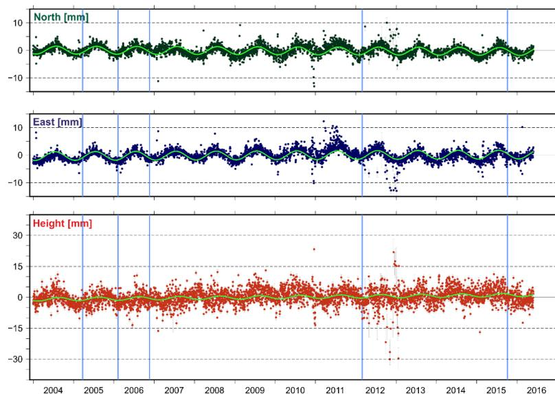
10 **Figure 5: Position time-series of the station KARL located in Karlsruhe, Germany.** Annual signals are well observed in the North and East components. Equipment change (indicated by the blue vertical lines) seems to be not affecting the time-series.
