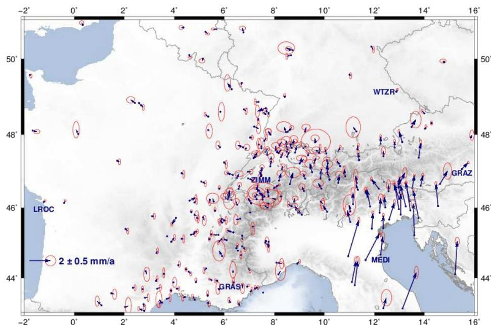
**Figure 7: Horizontal station velocities relative to the Eurasian plate with 95% error ellipses.** Labels identify the reference stations used for the geodetic datum definition: GRAS (Caussols, France), GRAZ (Graz, Austria), LROC (La Rochelle, France), MEDI (Medicina, Italy), WTZR (Bad Koetzing, Germany), ZIMM (Zimmerwald, Switzerland). Topography and bathymetry after the ETOPO1 model (Amante and Eakins, 2009).
