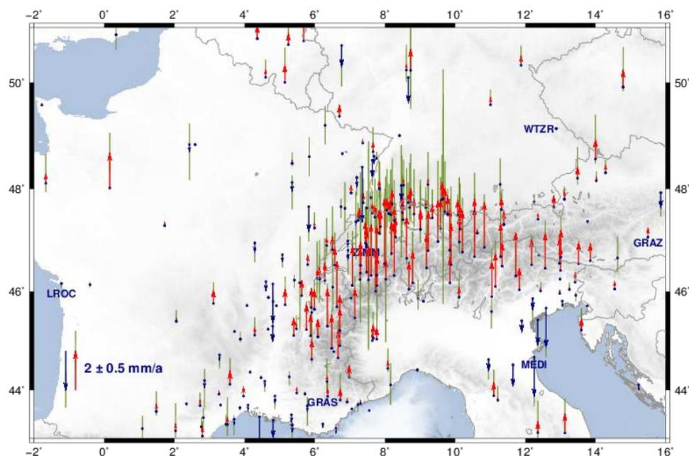
**Figure 8: Vertical station velocities:** Red arrows indicate uplift, blue arrows represent subsidence, green bars show 95% confidence. Labels identify the reference stations used for the geodetic datum definition: GRAS (Caussois, France), GRAZ (Graz, Austria), LROC (La Rochelle, France), MEDI (Medicina, Italy), WTZR (Bad Koetzing, Germany), ZIMM (Zimmerwald, Switzerland). Topography and bathymetry after the ETOPO1 model (Amante and Eakins, 2009).
