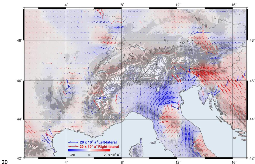
**Figure 15: Shear strain distribution in the Alpine Region.** Blue and red shades represent the left-lateral and right-lateral shear, respectively. For illustration purposes, the left-lateral shear is considered as negative and the right-lateral as positive. Topography after the ETOPO1 model (Amante and Eakins, 2009).
