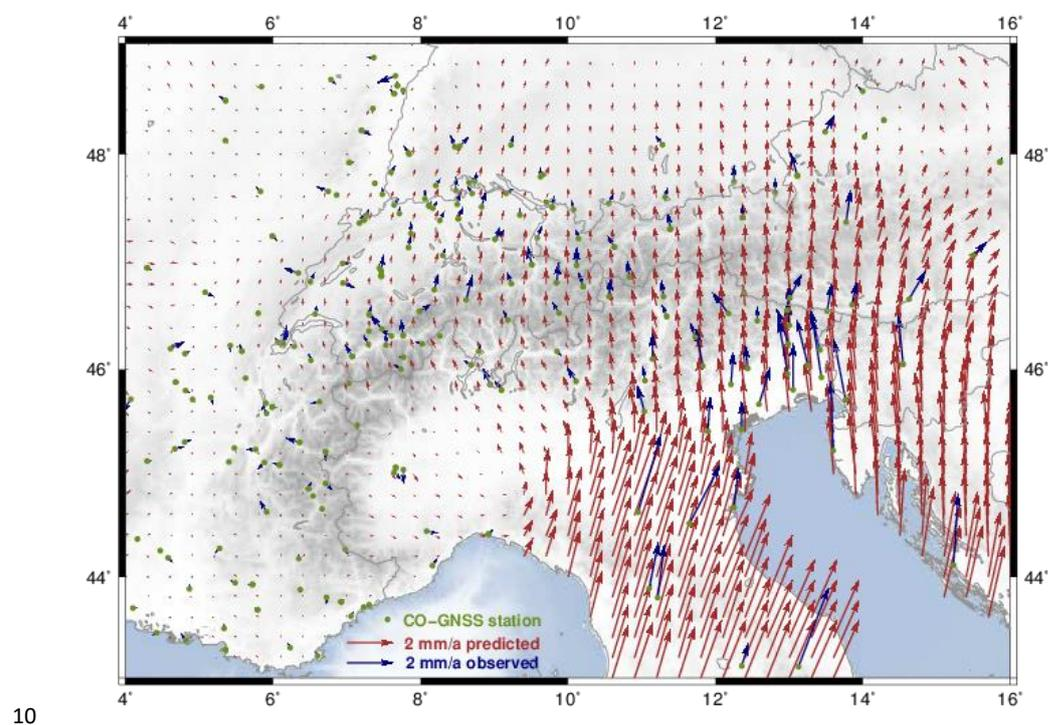
10 **Figure 9: GNSS-inferred horizontal deformation model of the Alpine region.** Red arrows represent the predicted surface deformation. Blue arrows represent the input residual velocities. Green dots show the CO-GNSS station distribution. Uncertainty ellipses are separately shown in Fig. 10. Topography and bathymetry after the ETOPO1 model (Amante and Eakins, 2009).
