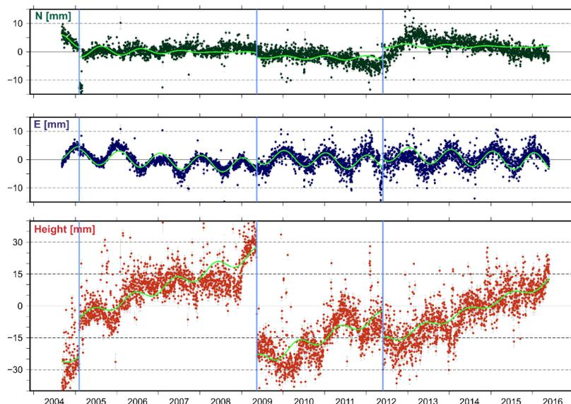
5 **Figure 4: Position time-series of the station BOLG located in Bologna, Italy.** Discontinuities (indicated by blue vertical lines) are caused by seismic events. Piecewise sinusoidal lines in light green represent a functional model approximating the seasonal motions detected at the station.
