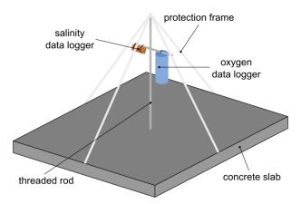
Figure 2. Scheme of deployed logger station
