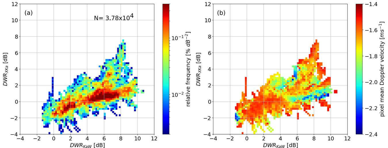
**Figure 12.** Triple frequency signatures for Level 2 data with temperatures between  $-20$  and  $-1$  °C and a mean Doppler velocity (MDV) above  $1.5 \text{ ms}^{-1}$  in order to select potentially rimed particles. Panel a shows the relative frequency of the observations; Panel b indicates the average MDV of each pixel in the histogram. Note the log-scale on the colorbar in A.
