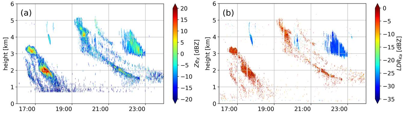
**Figure 6.** Time-height plots of the  $Z_{eX}$  and  $LDR_{Ka}$  of 23.11.2015 between 16:00 and 23:59. The region where the LDR is  $\approx -5$  dB is most probably a results of chaff. The Ka Band software applies a filtering for non-meteorological targets which removes most of the chaff; only the filtered Ka Band data are included in the TRIPEX dataset. Note, that no such filtering is applied to the X Band and W Band data.
