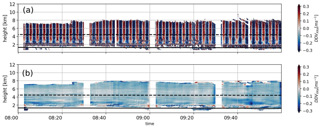
**Figure 7.** Time-height plots of the dual mean Doppler velocity using the Level 2 data of 20.11.2015. The dashed line and the continuous line are the  $-15$  and  $0$  °C isotherms, respectively. Panel a shows the  $DDV_{XKa}$  using the original data from Level 2. Panel b shows the  $DDV_{XKa}$  after applying a 3 minutes moving average.
