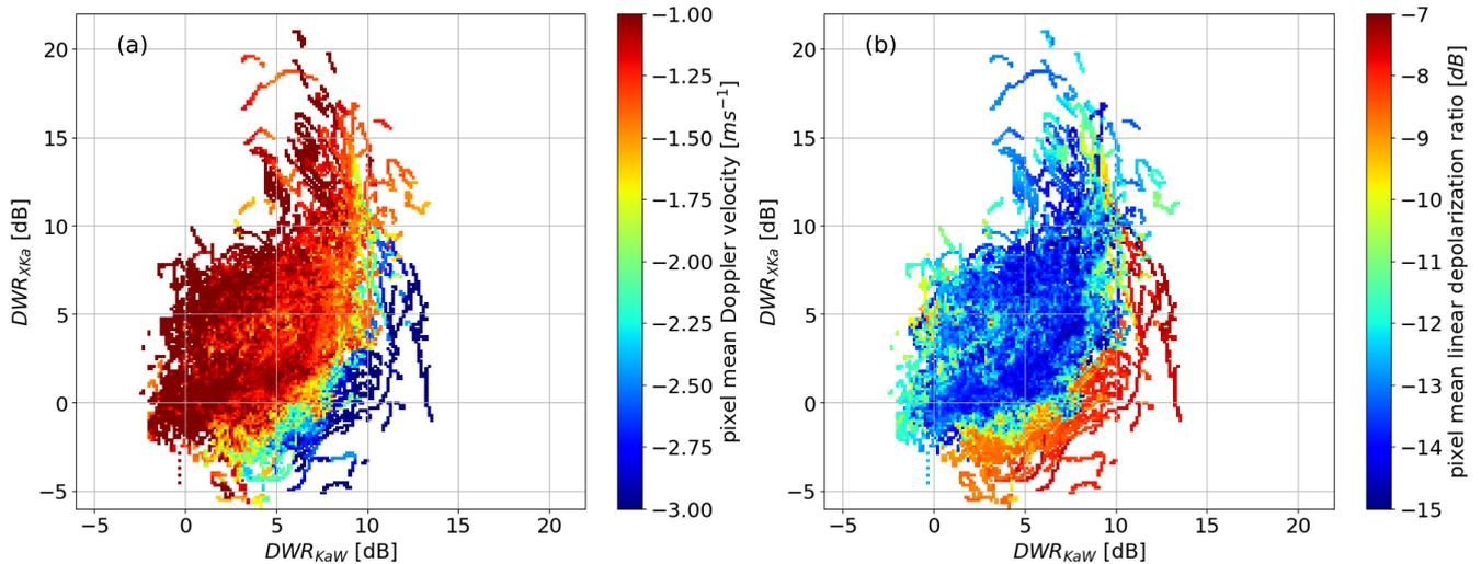
**Figure 13.** Triple-frequency diagrams of observations between 0 °C and the LDR maximum in the melting layer (same as Panel c of Figure 10), but the color in Panel a indicates the average MDV while in Panel b the color shows the average LDR.
