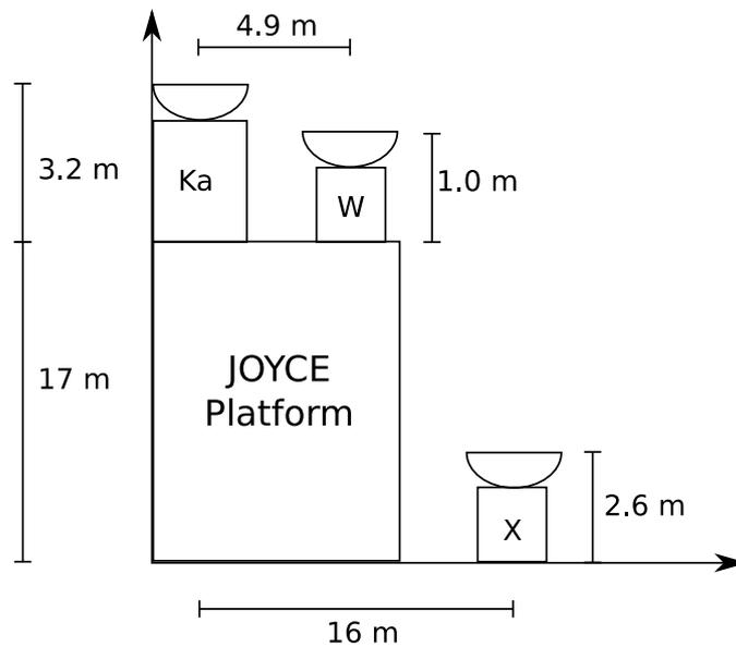
**Figure 1.** Sketch (not to scale) of the horizontal and vertical distances between the three zenith-pointing radars operated during TRIPEX. The JOYCE-CF platform with all auxiliary instruments is located on the roof of a 17 m tall building. The mobile X Band radar was placed on the ground close to the other two radars.
