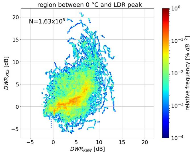
**Figure 11.** Two dimensional histogram of the triple frequency signatures for the region between 0 °C and the LDR maximum in the melting layer normalized by the total number of points  $N$ . The color shows the relative frequency and the binning is matching what has been used for Figure 10. Note the log-scale on the colorbar.
