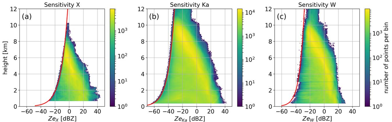
**Figure 8.** Histograms of reflectivities from the entire TRIPEX campaign Level 2 data for each radar. The red curve is the profile of the minimum retrieved reflectivity (Eq. 2). Panels a, b and c show the histograms for X, Ka and W Band, respectively; all error flags (see Tab. 4) were applied to filter the data. Note the log-scale on the colorbars.
