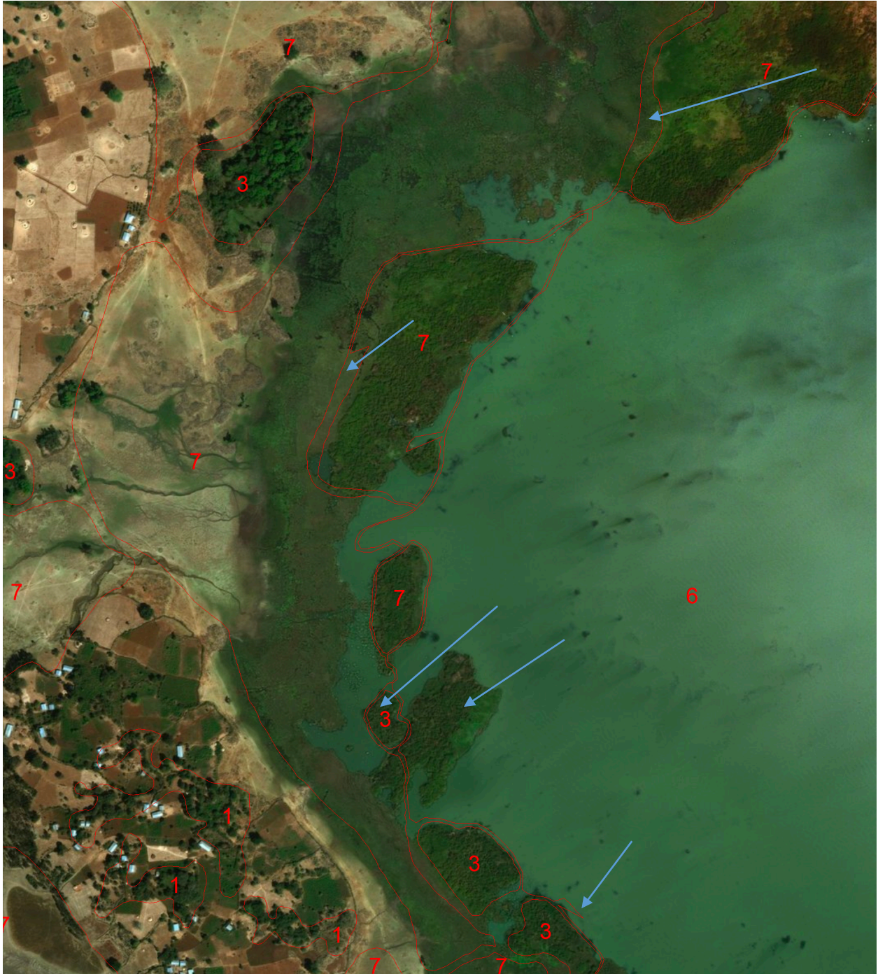
Fig 2. Gaps and classification accuracy. Map is on ArcMap 1:5000 scale. Arrows from the top to bottom indicate: the 1st and 2nd: unnecessary gaps between class 7 (wetlands); the 3rd, miss classification between 3 (natural forest) and 7; the 4 th , unidentified island; the 5 th , boundary error.
