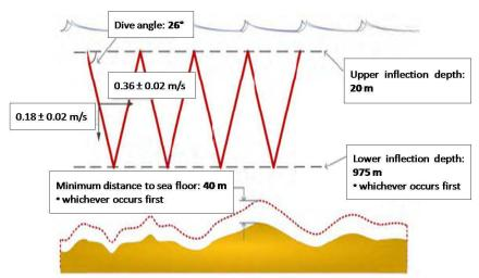
Figure 3. Glider navigation scheme during the ABACUS missions. The upper inflection depth was changed after the ABACUS 2014 mission in order to allow the glider reaching the surface at every second profile.
